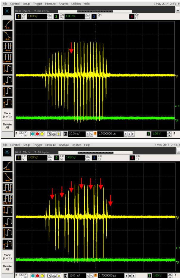
Figure 6: With an initial fill of 20 consecutive bunches, bunches at arrow locations were knocked out using vertical plane bunch excitation. (top) bunch #9 was kicked out; (bottom) bunches were kicked out every three buckets.
