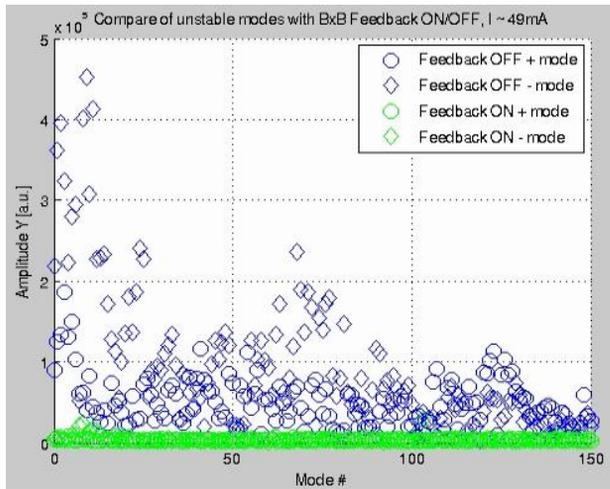
Figure 7: Comparison of vertical mode amplitude with and without bunch-by-bunch feedback.
