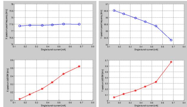
Figure 4: Transfer function spectrum peak frequency and 3dB bandwidth change at different single bunch current.
