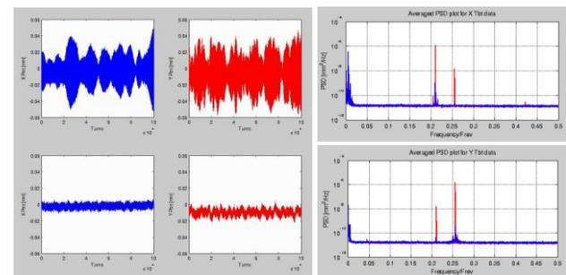
Figure 5: (left) BPM X/Y TbT data from one of the storage ring BPM C30BPM1; (right) BPM TbT data spectrum averaged from 180 BPMs, red traces were spectrum with bunch-by-bunch feedback OFF and blue traces with feedback ON.
