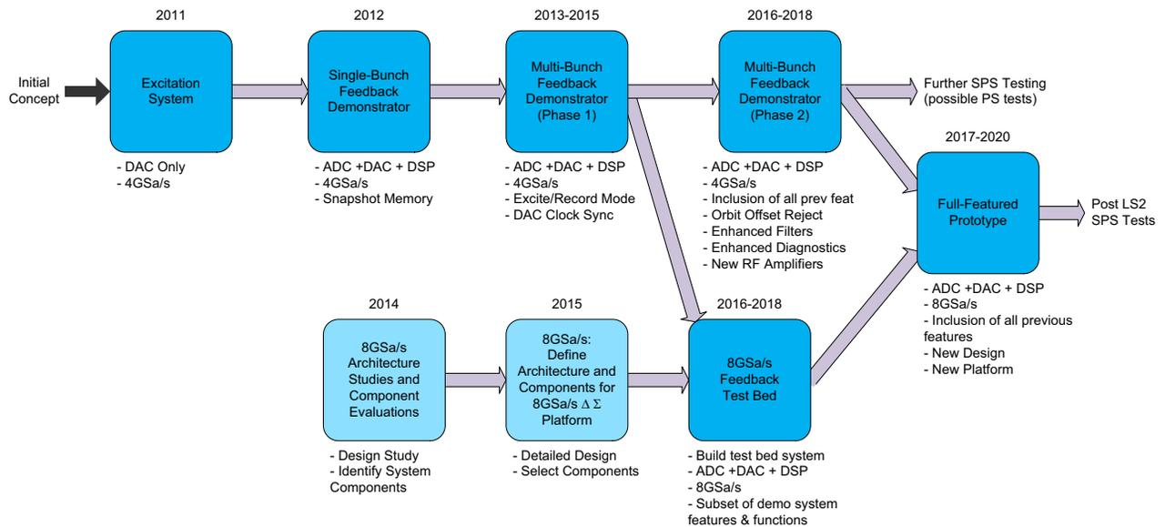
Figure 2: The technology development plan for the LARP Wideband Feedback effort, showing the path of expansion of the Demonstration system, and a parallel technology path with a higher sampling rate. We anticipate that the operational experience from the demonstrator system will guide the features to be implemented in the full-featured prototype in 2017.
