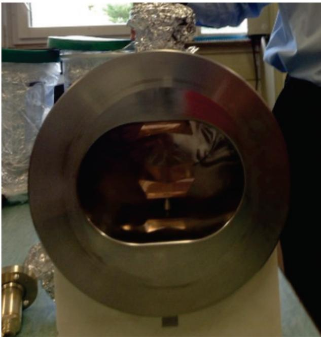
Figure 3: The first completed stripline kicker module for installation in SPS. The beam line vacuum system has been developed to allow 3 stripline kickers, as well as two slotline kickers, for beam testing. Dummy vacuum sections are in place to allow rapid and efficient installations of the third stripline kicker and a future slotline kickers. charge) as part of the computation of a correction signal.
