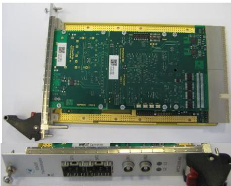
Figure 15: New PMC-FPGA board from IOxOS (side and front views).
