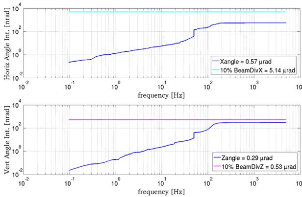
Figure 7: Beam angle stability at source point wrt specification of 10% of beam divergence.
