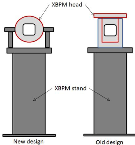
Figure 2: X-BPM head (in red) and stand in old and new designs. Whereas the old X-BPM head was plunging into the vacuum chamber, the new one is supported by a cradle and presents an axial symmetry to cancel the thermal expansion effect in the position calculation.
