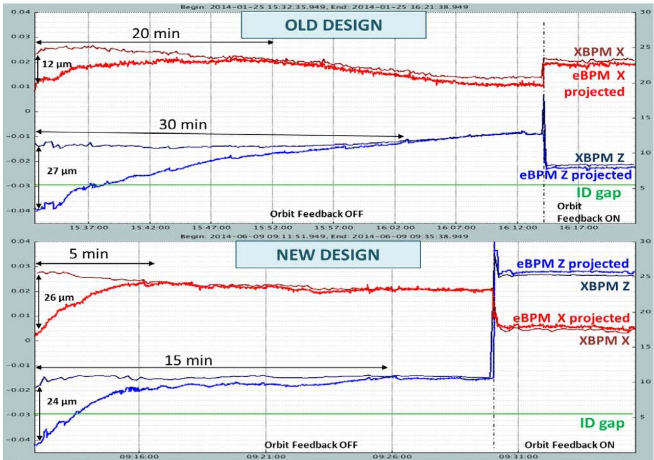
Figure 6: Stability comparison of the Nanoscopium X-BPM: (Up) for the old design and (bottom) for the new design in both horizontal and vertical plane. Stabilization time of the measurement after an injection from 0 to 430 mA has been reduced in both planes with the new design.
