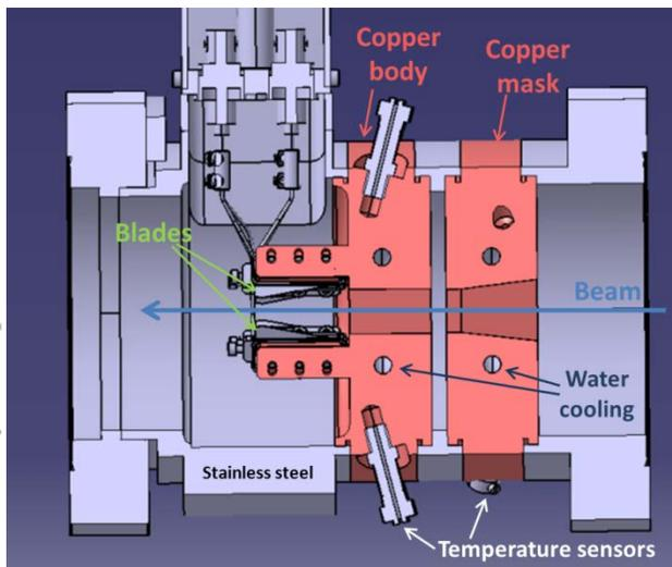
Figure 3: Different pieces of the X-BPM head: mask and body are both made of copper but separated to avoid thermal exchanges. A water cooling circuit is used to extract heat load.
