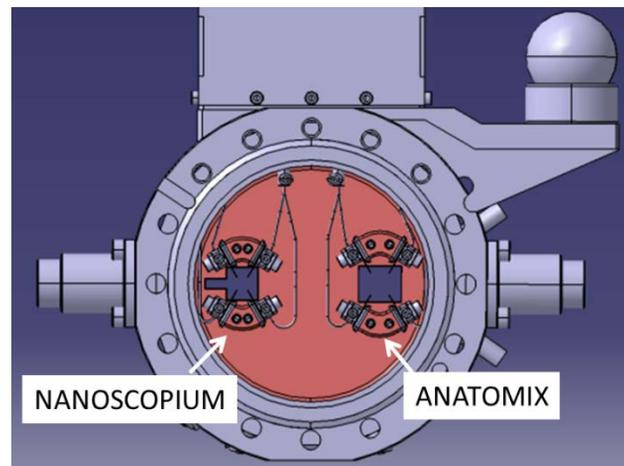
Figure 5: Double unit X-BPM head that has been manufactured for testing on the canted Anatomix and Nanoscopium SOLEIL beamlines.
