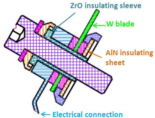
Figure 4: The stack made for blade insulation preserves a good thermal conductivity to extract the heat load deposited by the beam on the blade.
