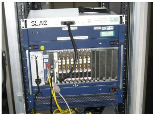
Figure 3: microTCA BPM system installed at PAL ITF.
