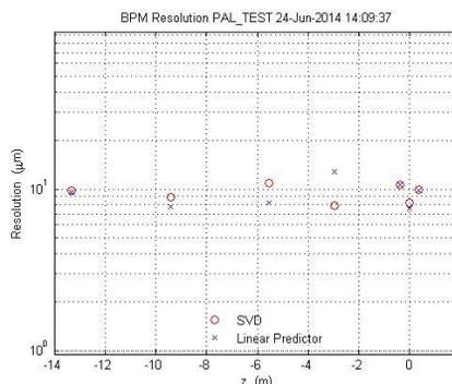
Figure 6: Multi-BPM resolution test at 10pC.
