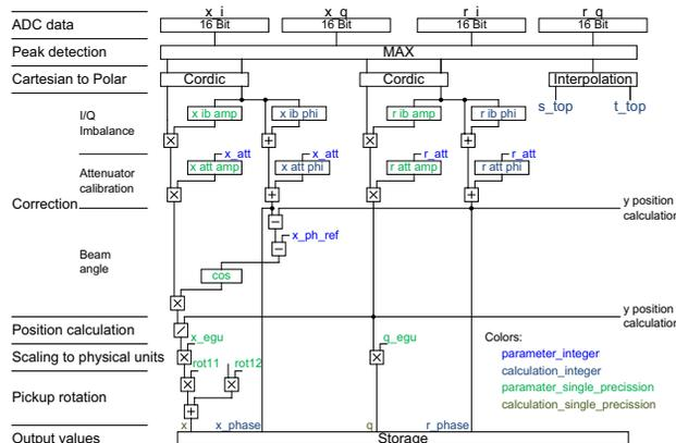
Figure 4: Simplified data flow of the CBPM signal processing algorithm.
