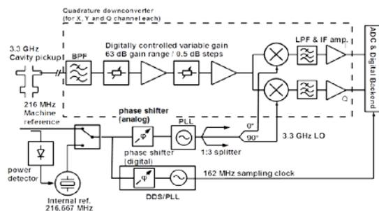
Figure 2: Simplified schematics of low-Q CBPM RFFE electronics, showing only one of its three input channels.
