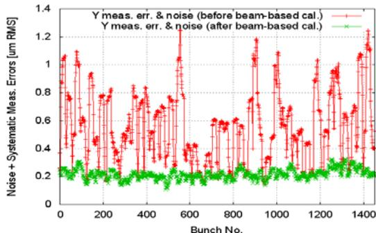
Figure 6: Floating average of the Y RMS measurement error (noise plus systematic errors due to switching attenuators etc). of FLASH CBPMs vs. bunch number before and after beam-based calibration of attenuators, calculated by correlating the readings of three CBPM10.
