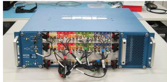
Figure 3: Cavity BPM electronics for two BPMs. Two RFFEs (top) and the FPGA carrier board with ADC mezzanines (bottom) are inserted into a customized crate from the front side. Power supply module and boards with SFP+ transceivers etc. are plugged in from the rear side.
