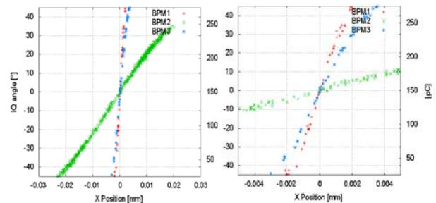
Figure 5: Measurement of IQ vector phase vs. beam position (same data with different X scales).
