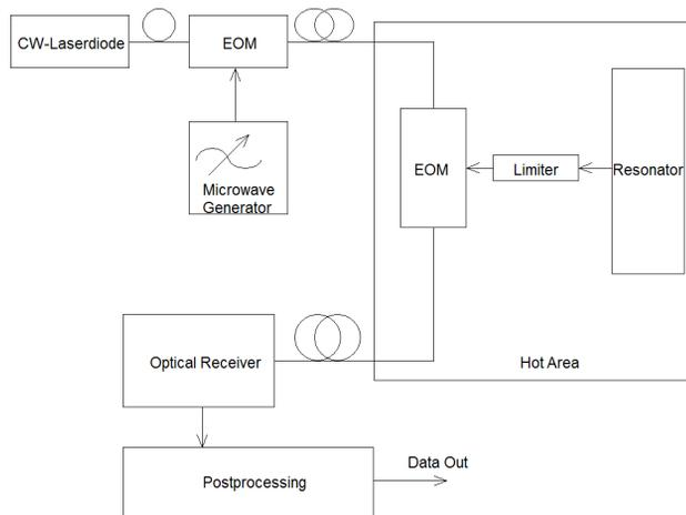
Figure 3: Layout of electro optical front end.
