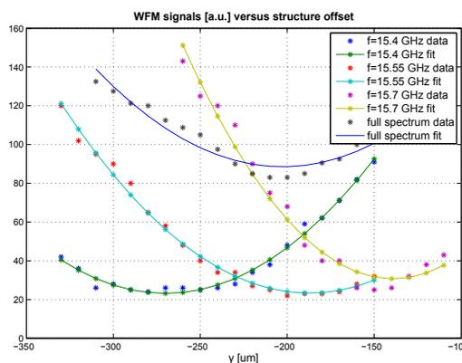
Figure 8: Spectral scan showing structure tilt, the curve with the full spectrum gives the average offset, while the filtered data shows the offset of different segment (15.4 GHz upstream end, 15.55 GHz near cell 18, 15.7 GHz in the middle of the structure).
