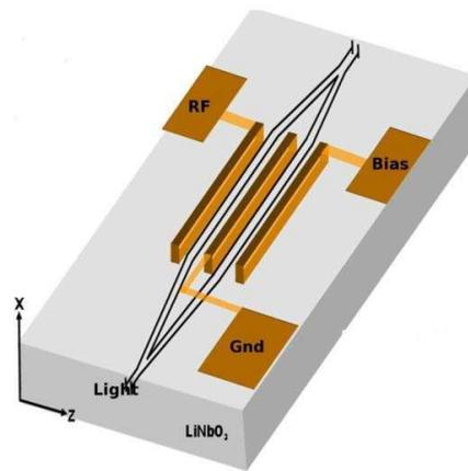
Figure 4: Electro optical modulator.
