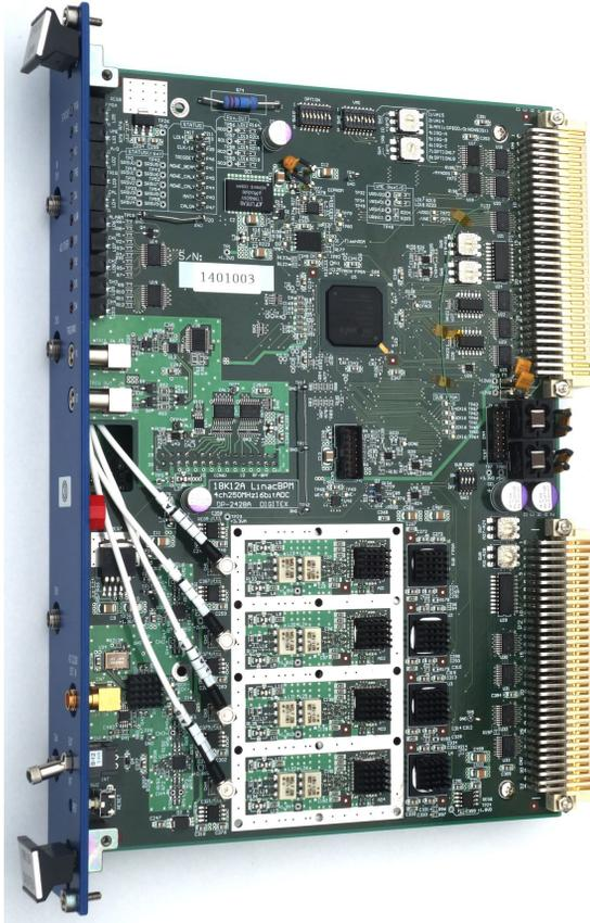
Figure 2: An photograph of prototype of BPM readout board (called 18K12A) is shown. This is a double width module. A BPF board is attached on bottom of a main (ADC) board. The output from BPF board is fed to the main board via four coaxial cables.
