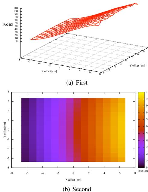
Figure 2: 3D and top view of the R/Q map of the simulated elliptical cavity in the region around the center of the beam pipe.
