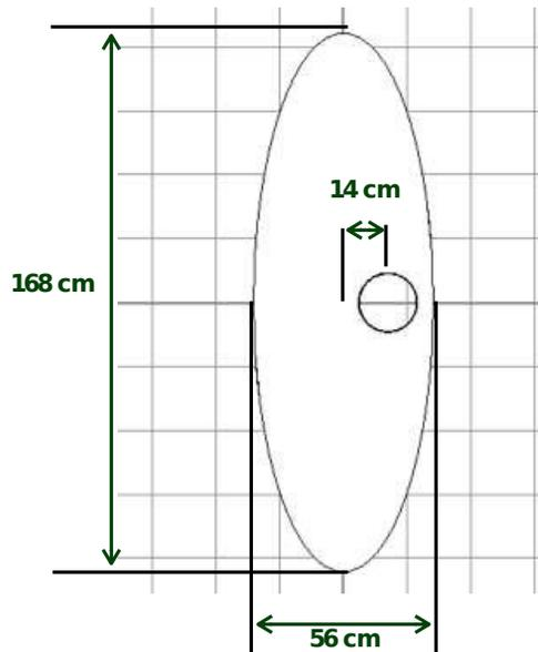
Figure 1: The simulated elliptical cavity.
