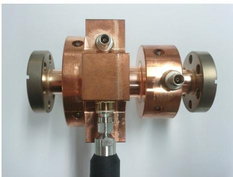
Figure 4: PAL XFEL RF X-band cavity BPM.
