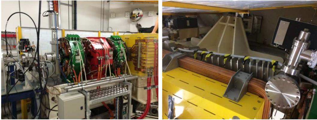
(a) Storage Ring scrapers (far left), Beam Loss Monitors behind dipole (far right). (b) Optical fiber installed in the outer side of the bending magnet, beam from left to right (top view).
