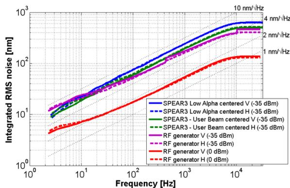
Figure 8: Integrated RMS position noise for four different conditions: (i) SPEAR3 beam in low alpha mode (200 mA), (ii) SPEAR3 beam during user shift (500 mA), (iii) RF generator R&S SMB100A at -35 dBm, and (iv) RF generator R&S SMB100A at 0 dBm.
