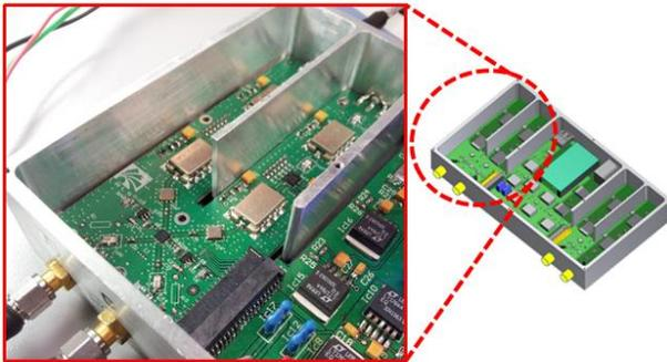
Figure 1: RFFE v2 prototype board. The dimensions of the prototype aluminum box are 20 cm x 11.5 cm.
