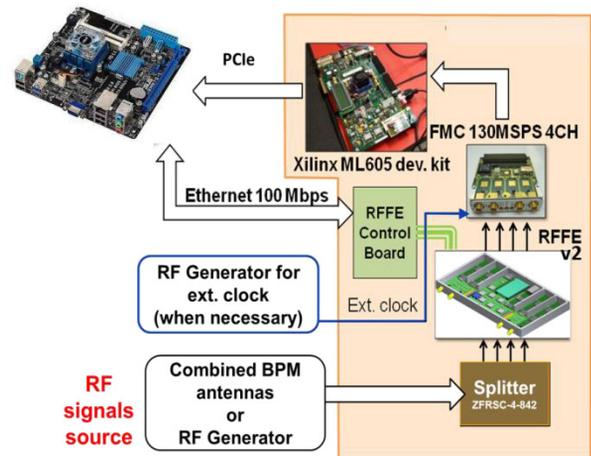
Figure 2: Block diagram of the setup used for the BPM electronics test.
