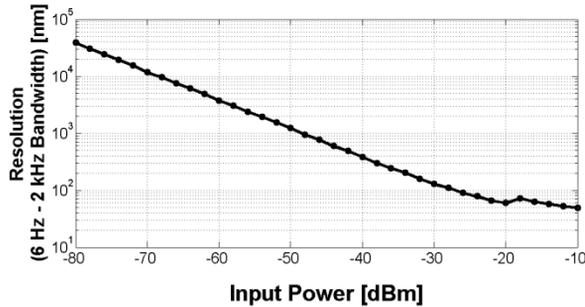
Figure 3: Resolution in function of input power.
