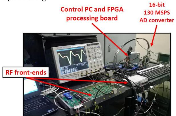
Figure 7: Setup used for the tests with beam at SPEAR3.
