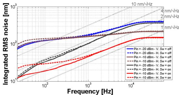
Figure 4: Integrated RMS noise for different input power and diagonal switching scenarios.
