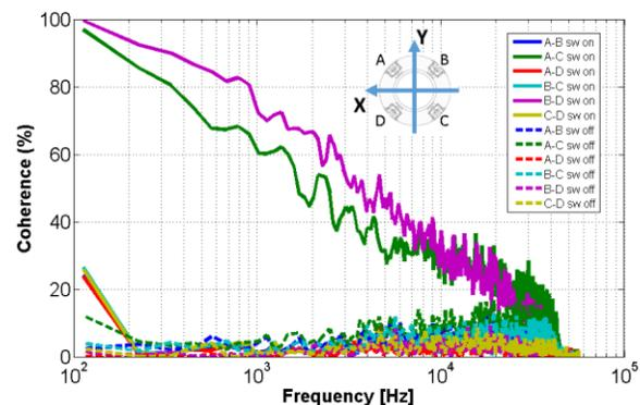
Figure 9: Coherence function between pairs of antenna baseband signal additive noise at FOFB data rate (~110 kHz). BPM signals naming convention is indicated.
