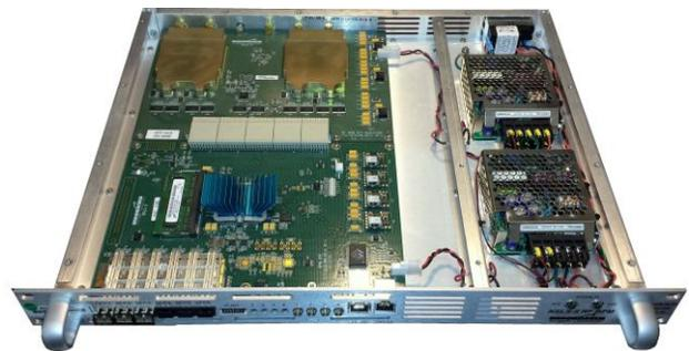
Figure 1: NLSL-II RF bpm electronics chassis.
