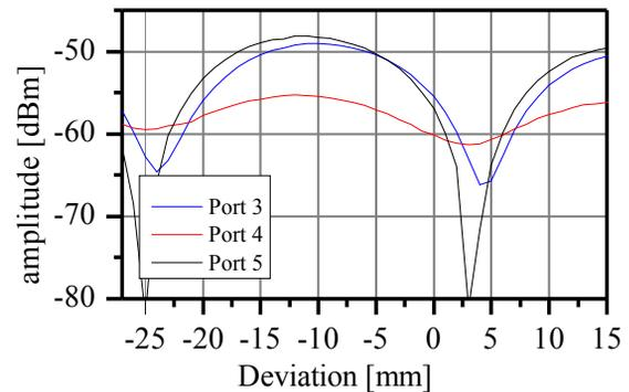
Figure 9: Detected power versus beam offset for ports 3,4 and 5 at a 3GHz.
