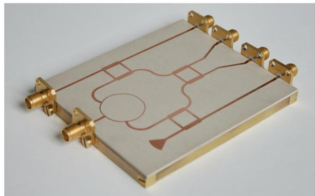
Figure 6: Photo of the six-port reflectometer design.
