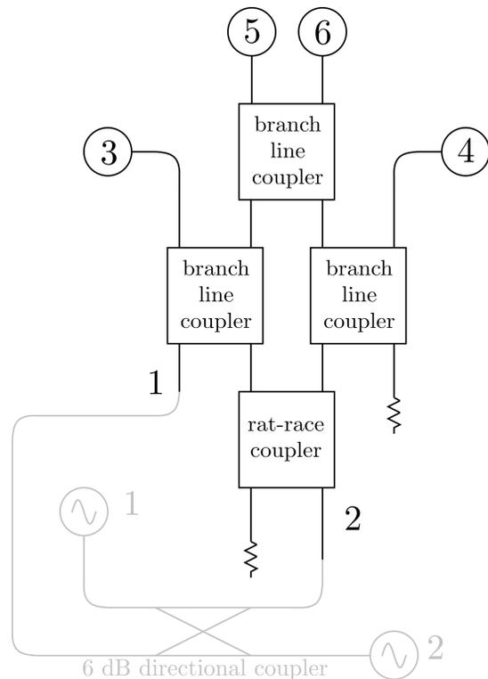
Figure 3: General circuit design for measurement purposes (Grey), and modified circuit design (black).
