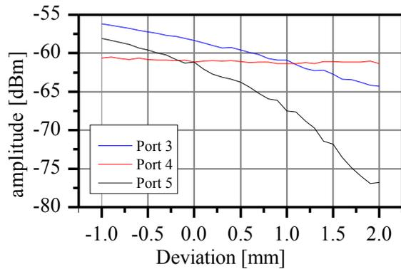
Figure 10: Detected power versus narrow beam offset for ports 3,4 and 5 at a 3GHz.
