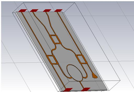
Figure 4: 3D model of the Six port reflectometer.
