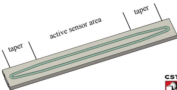
Figure 2: Simulation model of the quasi-grounded CPW structure.
