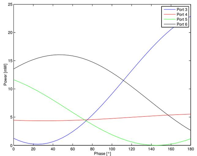
Figure 5: Output power versus phase difference of the six-port reflectometer.
