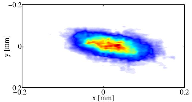
Figure 2: Transverse intensity distribution of the 38 nm HHG seed beam used at the direct seeding experiment sFLASH.
