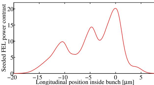
Figure 5: Power contrast along the internal bunch coordinate  $s$ .
