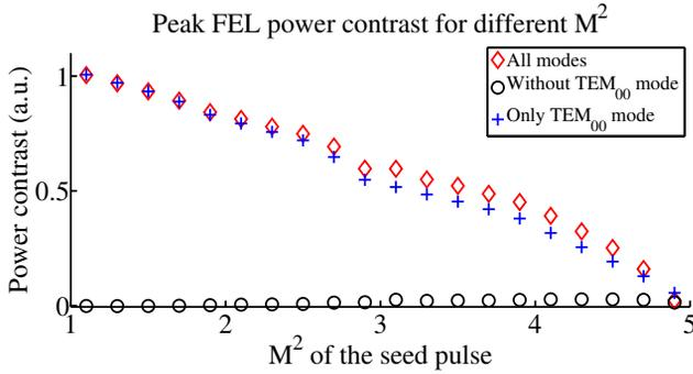
Figure 1: Seeded FEL power contrast vs.  $M^2$  of the seed pulse.
