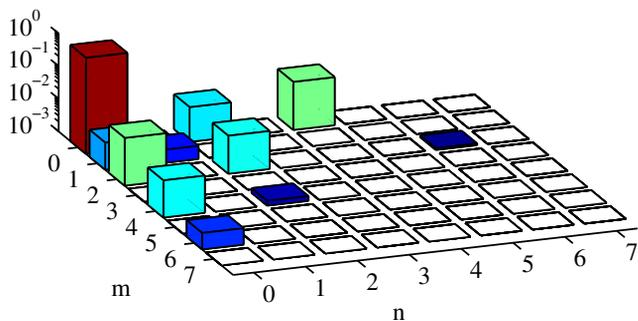
Figure 3: Power content coefficients  $c_{nm}$  of the harmonics beam shown in Fig. 2. The TEM<sub>00</sub> mode is with around 90% of the overall intensity the strongest mode. Power content coefficients smaller than  $10^{-3}$  are colored white.
