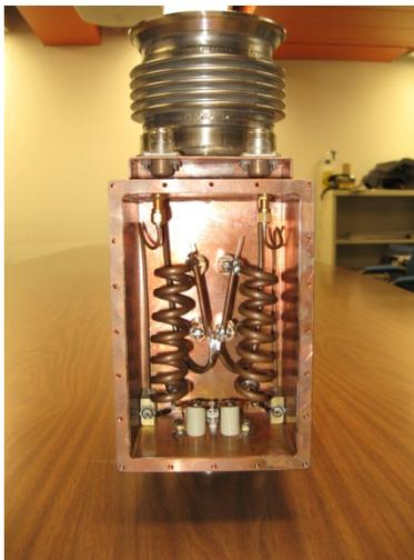
Figure 4: Short BPM detector (2).
