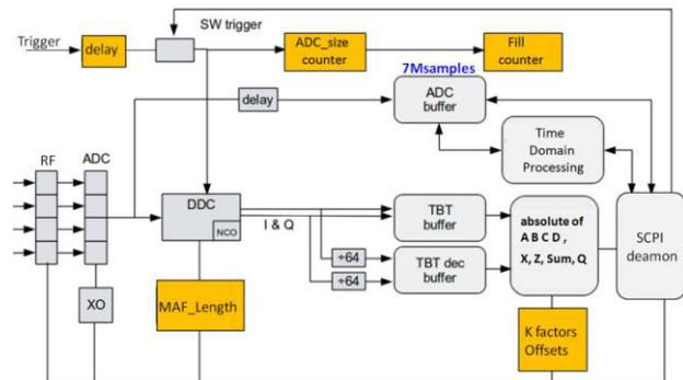
Figure 2: Signal Processing Scheme, the orange blocks indicate input parameters.
