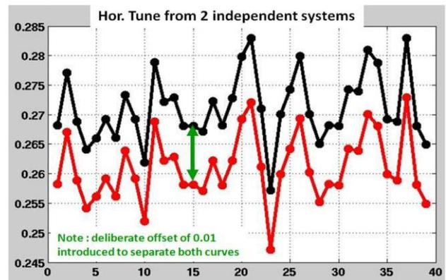
Figure 6: The horizontal tune stability, measured by 2 independent BPMs, over 40 shots at 4ms after injection.
