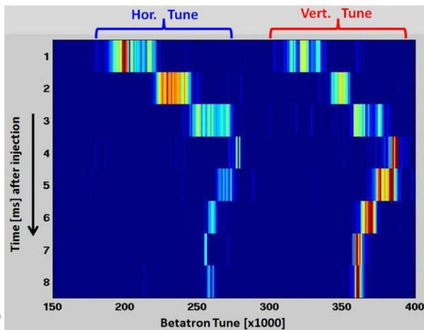
Figure 5: The tune behaviour in both planes of the injected beam during the first 8ms, in 8 slices of 1ms.
