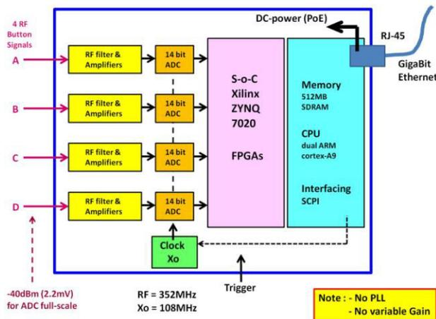
Figure 1: Block diagram of the Spark [um].
