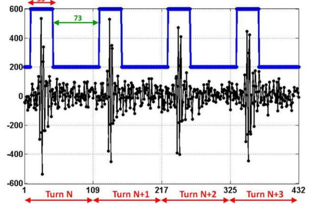
Figure 3: MAF filtering on the digitized RF signal with partial beam fill patterns (in this case single bunch).
