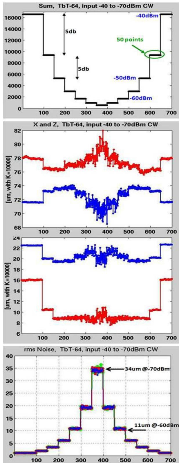
Figure 4: recordings over 23min showing from top to bottom values of Sum (i.e. Signal Level), X (blue) and Z (red) of both units, and rms noise. All data taken from the 16KHz rate buffers and with CW RF power at inputs, and with K-factor at 10mm.
