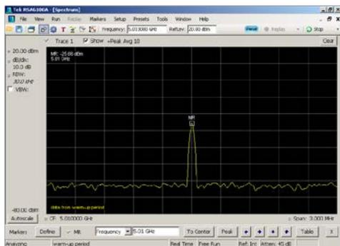
Figure 17: Signal input power at mixer (proportion 1/10).
