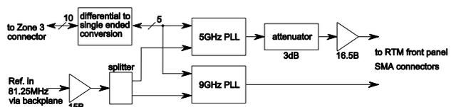
Figure 6: HOM PLL block diagram.
