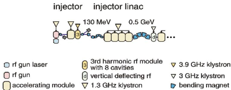
Figure 2: Schematic layout of the European XFEL injector [1].
