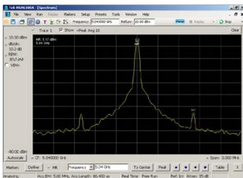
Figure 9: HOM-PLL 5GHz output.
