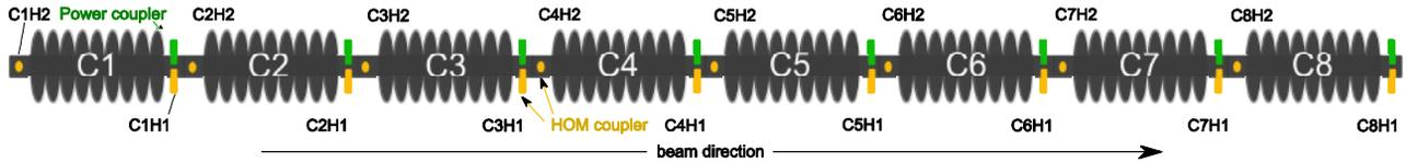
Figure 3: Cavity arrangement inside the module.
