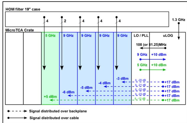
Figure 1: Overview over the complete system installation.
