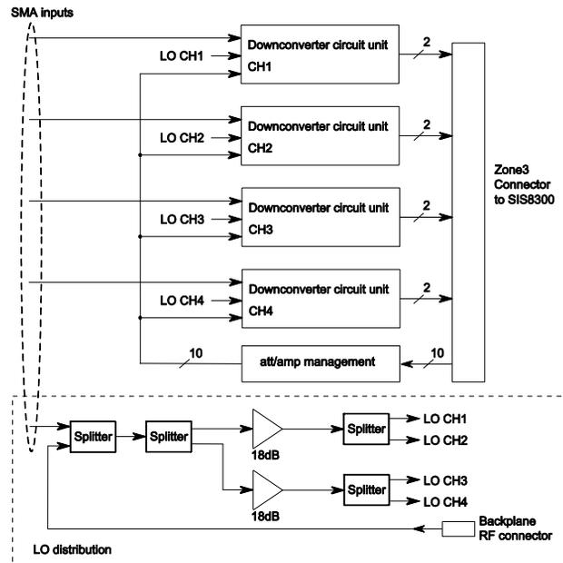
Figure 11: Block diagram of a downconverter card.
