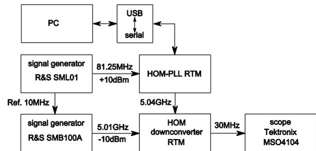
Figure 15: HOM downconverter test setup.
