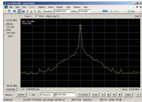
Figure 10: HOM-PLL 9GHz output.
