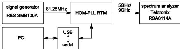
Figure 8: HOM-PLL RTM test setting.
