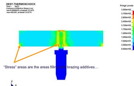
Figure 2: Thermo shock-analysis during cold/warm phases, stress of pin/ceramic/shell material (Novicos, Hamburg).
