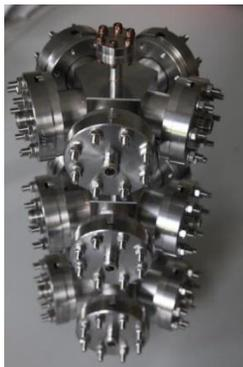
Figure 3: Vacuum test adapter for cryogenic tests under vacuum with continuous leak check in a vertical cryostat.
