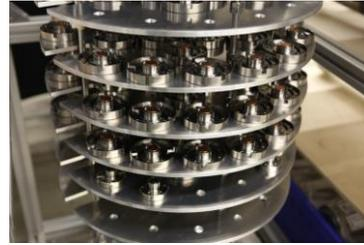
Figure 4: Multilayer table to "cryogenic-check" the serial production of feedthroughs.
