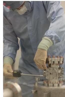
Figure 5: Assembling of feedthroughs with torque wrench in classroom class 4.
