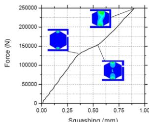
Figure 6: The deformation of the gasket cross section is shown. First step is the elastic to plastic zone. The distribution of equivalent plastic strains is shown at three different levels for alloy Al 5754.
