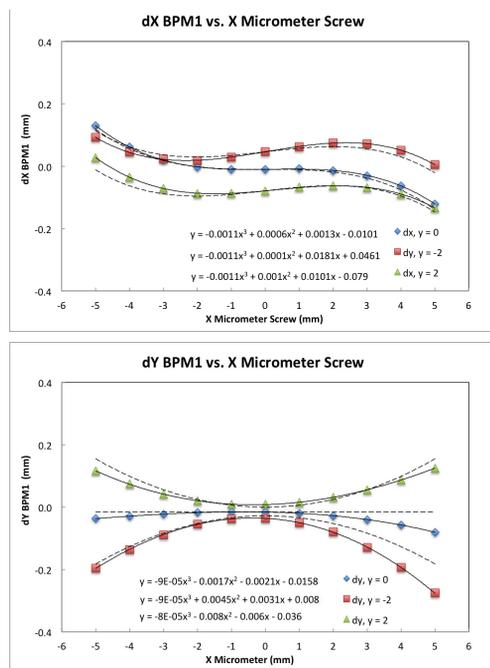
Figure 2: Deviation of the measured (calculated) BPM readout from the true position as a function of the wire position. Top figure: deviation in x for x movements for three y values. Bottom figure: deviations in y. Also shown is a 3rd order polynomial fit to the data.
