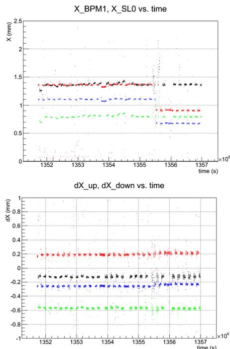
Figure 3: Top: Upstream horizontal Libera and Neumann BPM positions as function of time for  $e^+$  and  $e^-$  beams (fall running period Oct. 2012 to Jan. 2013.) Bottom: Difference of Neumann and Libera horizontal positions vs. time. Data are from the DORIS accelerator archive.
