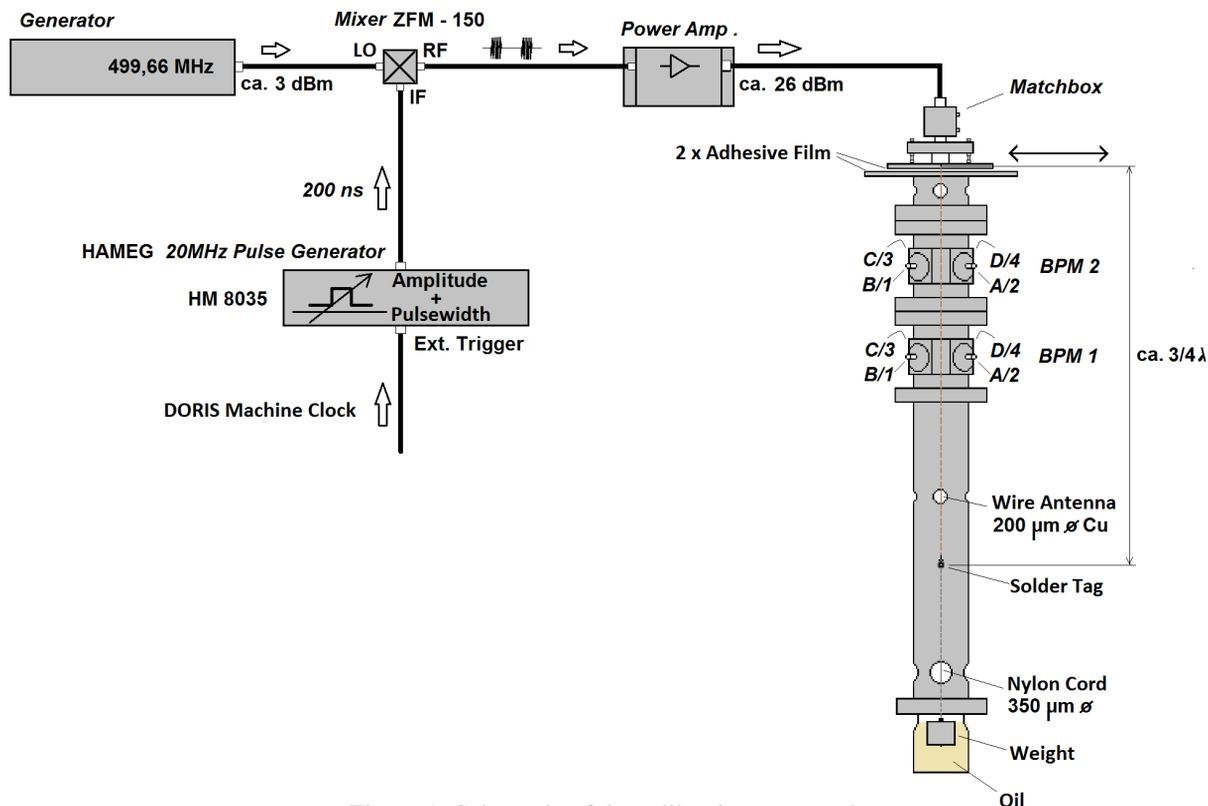
Figure 1: Schematic of the calibration test stand.
