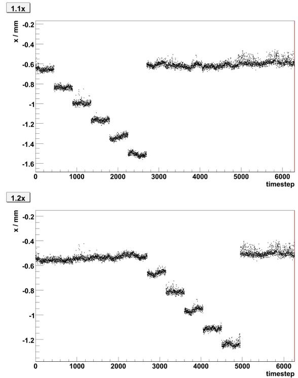
Figure 4: Position readings for different mover positions in  $x$  for first (1.1x) and second (1.2x) CBPM.
