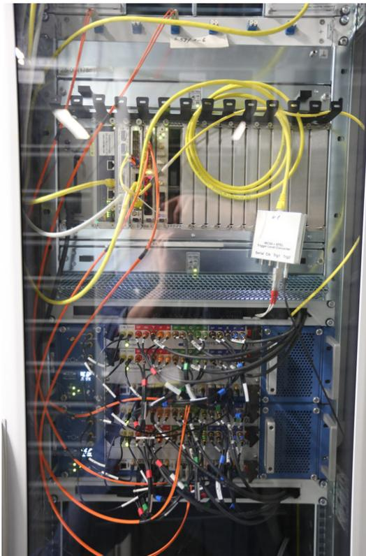
Figure 9: Undulator electronics for FLASH2 provided by PSI at the bottom part with 4 front-ends. Above is a  $\mu$ TCA crate with an FPGA/SFP board for the communication between PSI electronics and FLASH control system via fiber optic multi-gigabit links.
