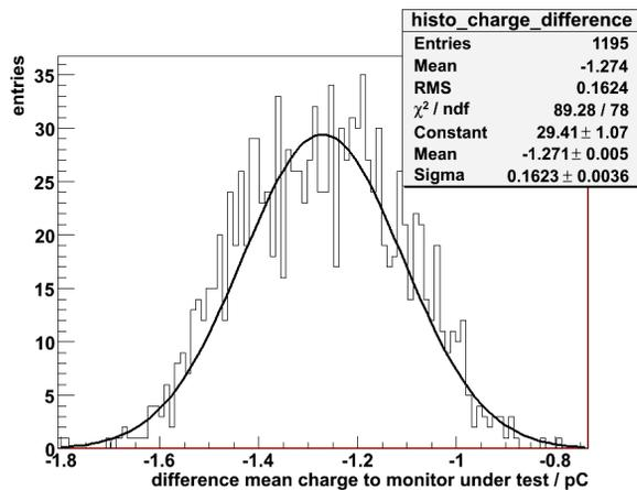
Figure 10: Difference between mean charge value to the monitor under test: here CBPM with the monitor number 19 with Gaussian fit at a charge of about 100 pC.
