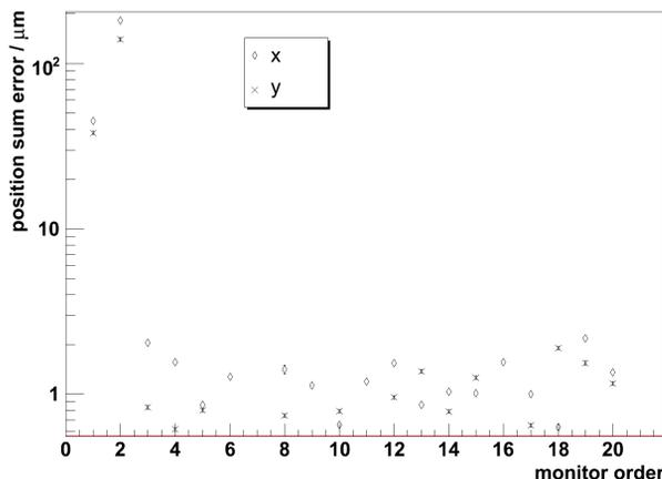
Figure 13: Sum error of BPM correlation at FLASH2 in both transverse planes for a charge of about 100 pC. The first two monitors are button BPMs, otherwise the order of CBPMs is similar to Fig. 11.
