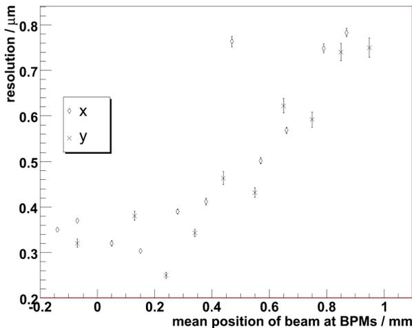
Figure 7: Resolutions of the undulator CBPMs at FLASH1 for different mean beam offsets in x and y for a charge of about 240 pC.
