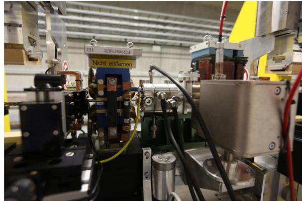
Figure 8: Undulator CBPM in an intersection of FLASH2.
