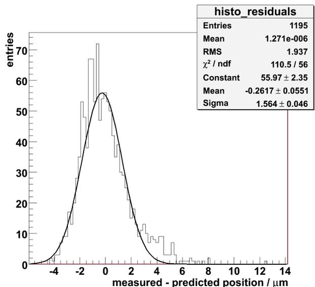
Figure 12: Difference between expected and measured position with Gaussian fit of a CBPM with monitor number 4 for position error calculation at the horizontal plane.
