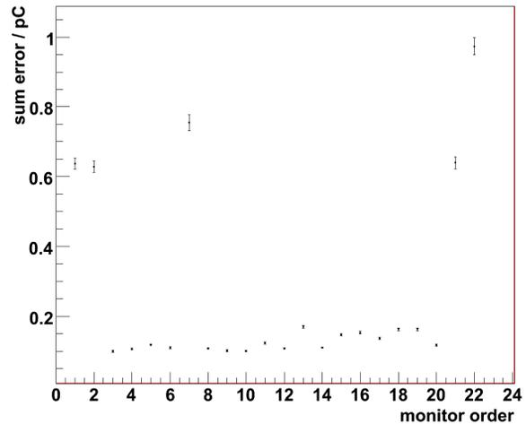
Figure 11: Sum of statistical and systematic errors of charge monitor correlation at FLASH2 at a charge of about 100 pC, with active automatic gain control of the CBPMs, ordered according beam direction. Values above 0.6 pC are from Toroids, values below from CBPMs.
