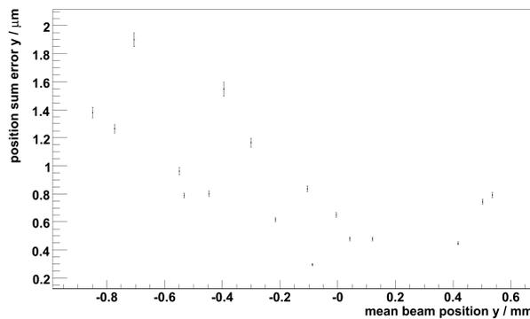
Figure 14: Sum error of CBPM correlation measurement at FLASH2 at the vertical plane with a charge of about 100 pC as a function of mean beam position.
