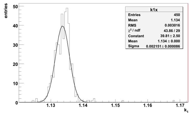
Figure 5: Histogram for different calculated correction values of first CBPM in horizontal direction with Gaussian fit.
