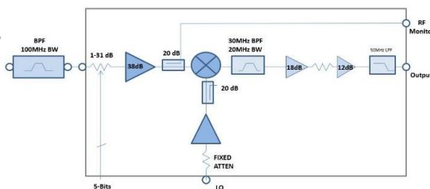
Figure 4: Block diagram of a downmix channel.
