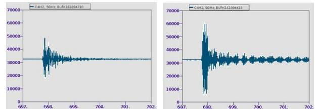
Figure 5: Raw signals from C1H2 (5 GHz channel) and C1H1 (9 GHz) from the control system.
