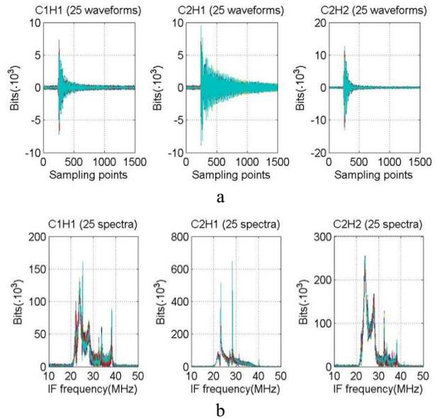
Figure 8: Waveforms (a) measured from three 9 GHz channels (C1H1, C2H1 and C2H2) and the corresponding HOM spectra (b) obtained by Fourier transform.
