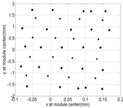
Figure 6: The beam positions as calculated at the module center from the two BPMs. One (larger) scan has been made for calibration data (dots), and another for validation data (stars).
