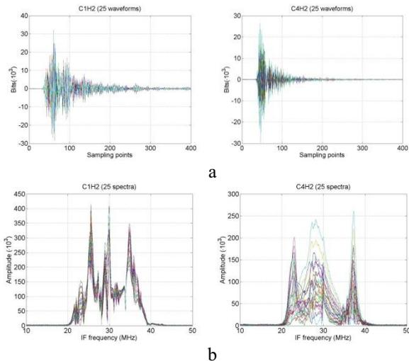
Figure 7: Waveforms (a) measured from the 5 GHz channels (C1H2 and C4H2) and the corresponding HOM spectra (b) obtained by Fourier transform.
