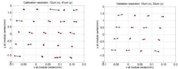
Figure 9: RMS errors obtained from calibration (left) and validation (right) data for the concatenated 5 GHz channels. Each beam position as interpolated from the BPMs (blue) is connected to the resulting position from the HOM signals (red).
