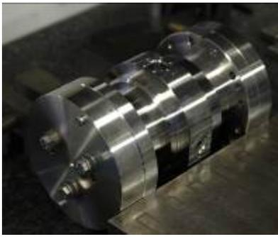
Figure 4: BPM mounted with its equipment used during EB welding.
