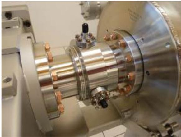
Figure 6: Re-entrant BPM mounted in an XFEL cryomodule.
