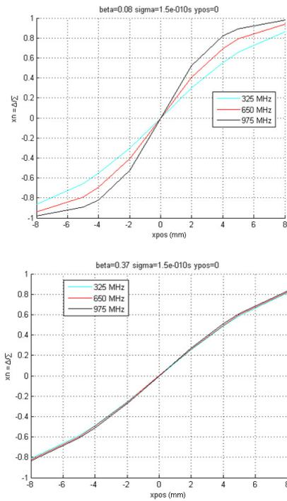
Figure 6: Horizontal beam position calculated using ‘delta-over-sum’ method at different frequencies with  $\beta = 0.08$  and  $\beta = 0.37$  for a bunch length = 150 ps. Vacuum aperture: 30 mm, button diameter: 14 mm.
