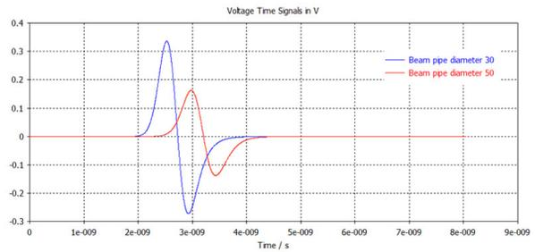
Figure 4: BPM output voltage for two different apertures used on the linac (bunch length 150 ps,  $\beta=0.37$ , 35 mA).
