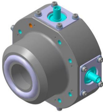
Figure 2: Design of the button BPM installed in the CH-inter-tank section.
