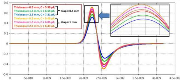
Figure 9: BPM output signals read by one electrode with different button geometries. Beam pipe = 30 mm, button diameter = 14 mm,  $\beta=0.37$  for a bunch length = 100 ps, 35 mA.
