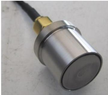
Figure 3: Kyocera button – diameter 14 mm.
