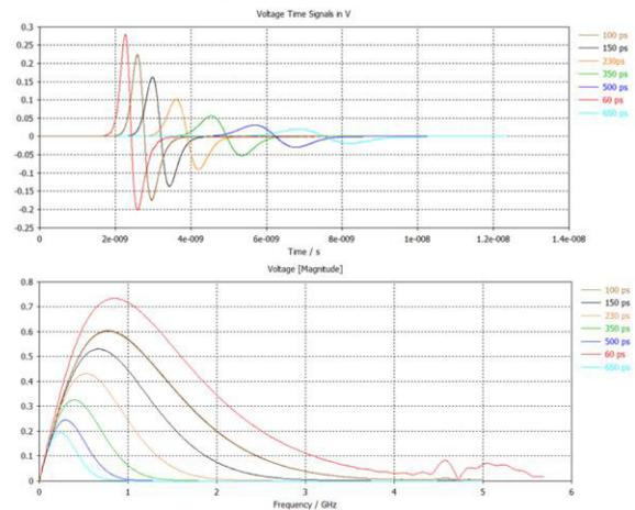
Figure 5: BPM output voltage for different bunch lengths beam pipe = 50 mm,  $\beta=0.37$ , 35 mA.
