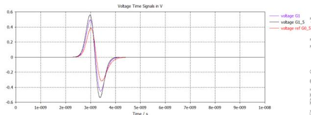
Figure 8: BPM output signals read by one electrode with the gap varying from 0.5 to 1.5 mm. Beam pipe = 30 mm, button diameter: 14 mm,  $\beta=0.27$  for a bunch length = 150 ps, 35 mA.
