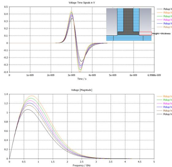
Figure 7: BPM output signals for different height of button given in units of mm. Beam pipe = 30 mm, button diameter: 14 mm  $\beta=0.27$  for a bunch length = 150 ps, 35 mA.
