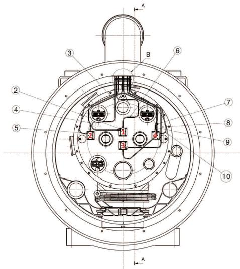
Figure 4: Cross section of an LHC dipole magnet showing the outer cryostat, the inner cold mass housing the superconducting coils and the position of cryogenic radiation detectors on the end of the cold mass.
