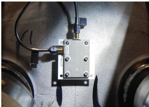
Figure 5: scCVD diamond detector mounted using a ceramic based holder.
