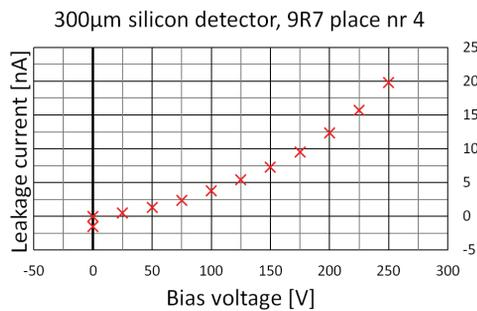
Figure 9: Leakage current of  $p^+ - n - n^+$  silicon radiation detector as measured in an LHC dipole magnet at a temperature of 295 K.
