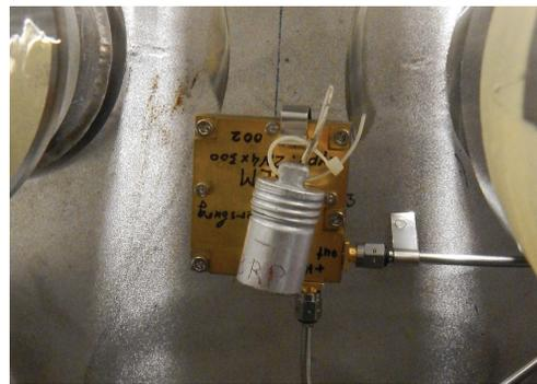
Figure 6:  $p^+ - n - n^+$  silicon detector mounted using an FR-4 glass-reinforced epoxy laminate based holder during testing with a gamma-radiation source (capsule).
