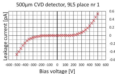
Figure 8: Leakage current of scCVD radiation detector as measured in a LHC superconducting dipole magnet at a temperature of 295 K.
