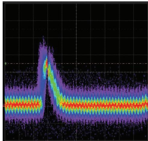
Figure 7: Beta-radiation induced signal from a scCVD diamond cryogenic radiation detector in the LHC magnet (80 mV on vertical and 40 ns on horizontal scale).
