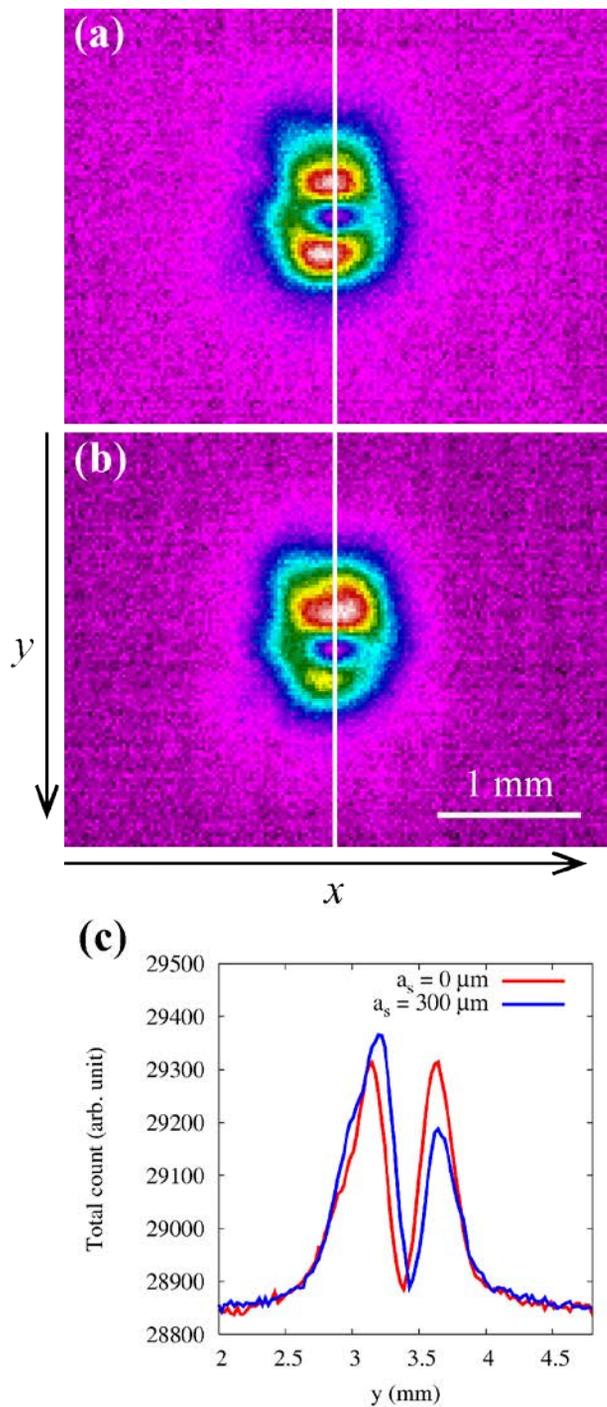
Figure 5: Spatial distribution of CDR measured with the terahertz camera. The electron beam trajectory offsets with respect to the slit center as (a) 0  $\mu\text{m}$  and (b) 300  $\mu\text{m}$ , respectively. (c) The line intensity distribution given in (a) and (b), respectively.
