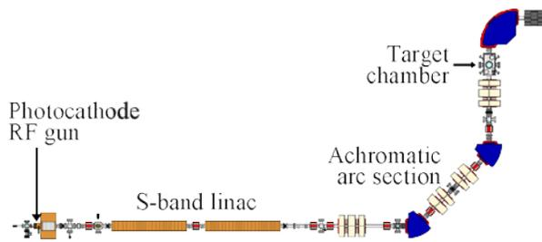
Figure 2: Schematic illustration of the S-band compact electron linac at AIST.
