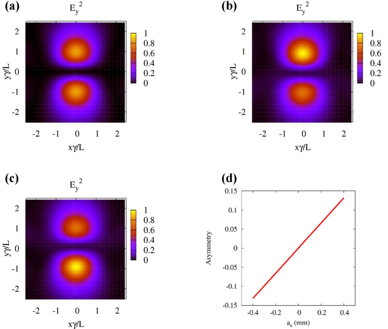
Figure 1: Normalized spatial distribution of vertically polarized DR calculated for different offsets of the electron beam trajectory with respect to the slit center derived from Eqs. (3) – (5). (a)  $a_s = 0.0$  mm, (b)  $a_s = -0.4$  mm, and (c)  $a_s = 0.4$  mm. (d) Asymmetry in the plane  $x = 0$ .
