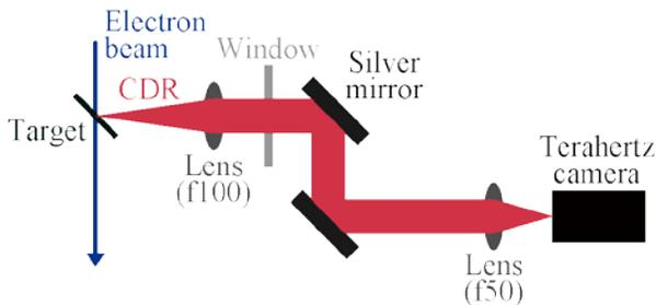
Figure 3: Schematic illustration of the spatial distribution measurement of CDR generated from the rectangular slit using the terahertz camera.
