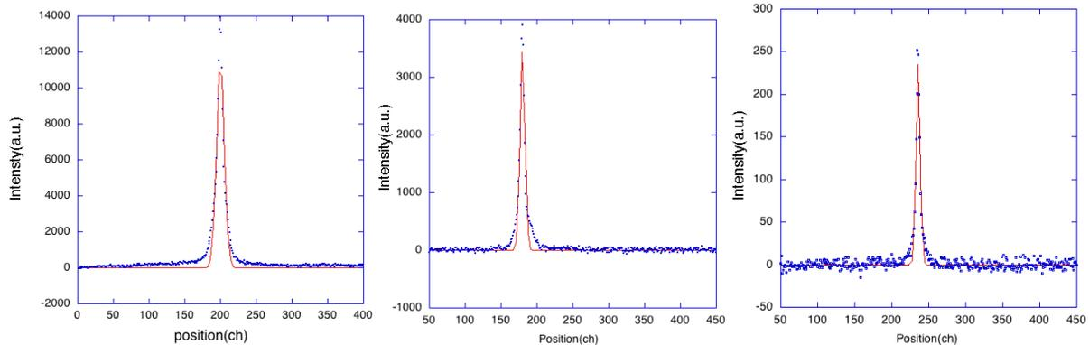
Figure 7: 1) Ceramic YAG:Ce 100µm thickness(left)  $\sigma_y=13.9\mu\text{m}$ , 2) Ceramic YAG:Ce 50µm thickness(center)  $\sigma_y=8.6\mu\text{m}$ , 3) Crystal YAG:Ce 50µm thickness(right)  $\sigma_y=7.0\mu\text{m}$ (right).
