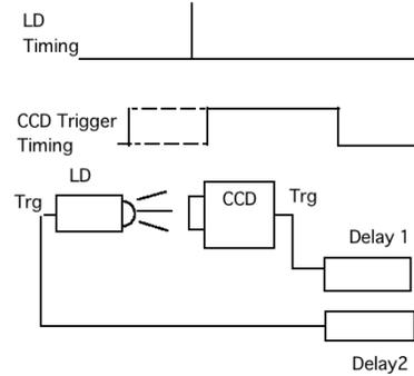
Figure 3: Measurement setup of the gate characteristics of the CCD.
