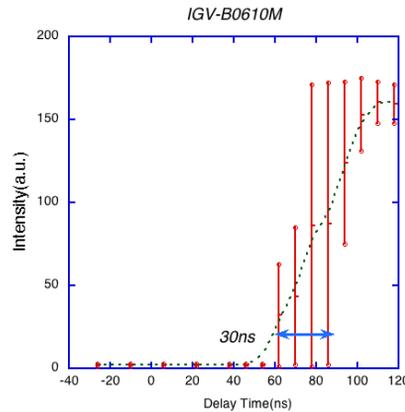
Figure 4: Gate characteristics of IGV-B0610M.
