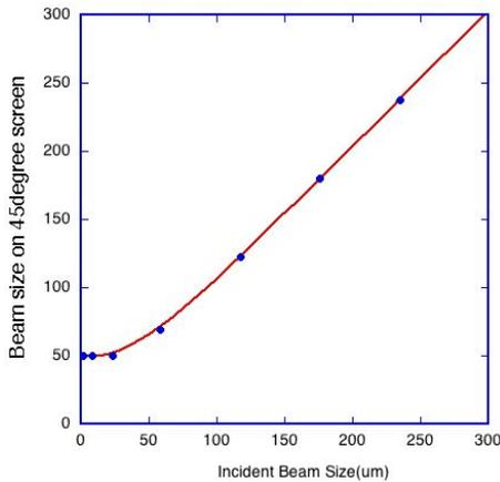
Figure 2: Calculation of the horizontal beam size at oblique angle of 45 degrees screen in the case of 50 $\mu\text{m}$  thickness.
