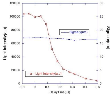
Figure 9: The scintillation light intensity and the measured vertical beam size as a function of the gate timing of the CCD.
