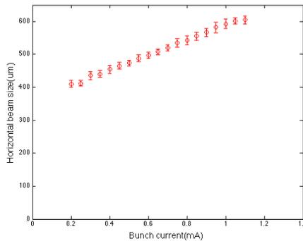
Figure 6: Current dependence of the horizontal beam size.
