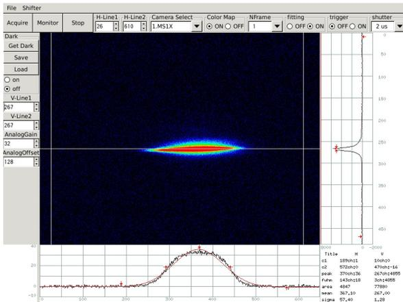
Figure 8: Example of the saturated beam profile.
