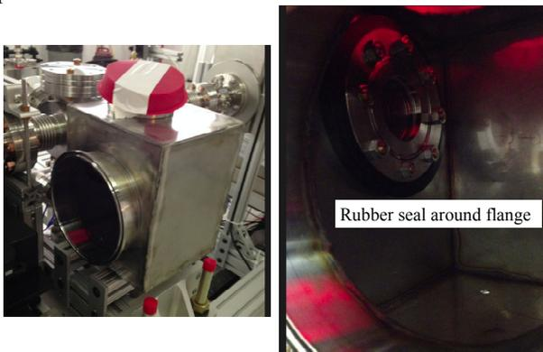
Figure 10: Stainless steel box mounted over flange on X121. Box is sealed around flange with a Uniseal gasket.
