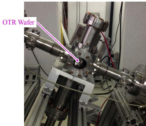
Figure 5: X124 cross in downward beamline to dump. There will be an optics system attached to this side of the cross.
