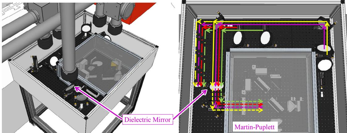
Figure 6: Left) 3-D model of OTIS box. Right) The colors indicate source, Yellow – X124, Purple and Red – Compressor, Green – X121. Solid lines go to the streak camera. Dashed lines go to the interferometer, Dot-Dash lines go to the user area in the box.
