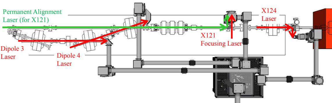
Figure 13: Laser paths for alignment purposes. Dipole 3 and 4 and X124 lasers will do both focusing and alignment.
