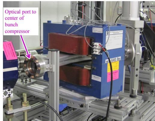
Figure 3: Second dipole in bunch compressor showing the optical entrance port to the center leg of the chicane. The beamline through the dipole is X shaped.
