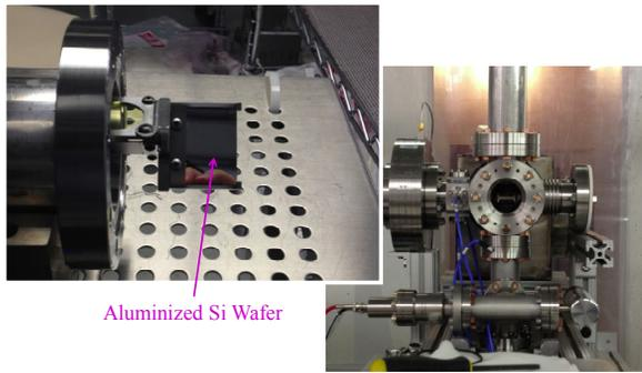
Figure 4: Left) X121 actuator retracted; OTR wafer is visible. Right) X121 cross with actuator installed.
