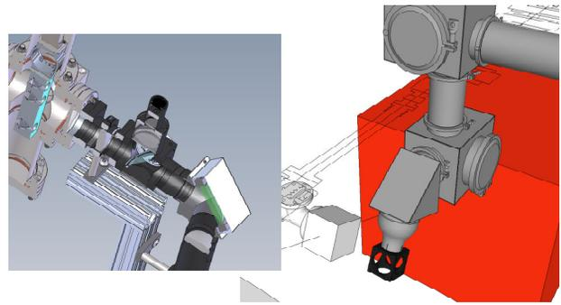
Figure 11: OTIS extraction from X124. Left) Normal camera optics cross section. Right) Attachment point of OTIS transport line.
