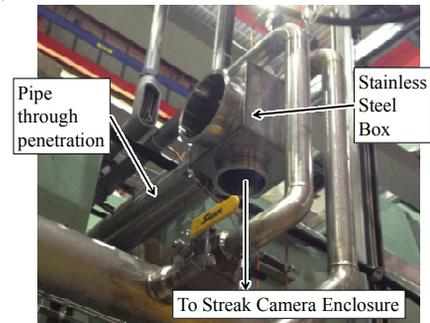
Figure 12: Penetration pipe and mirror box before the streak camera.
