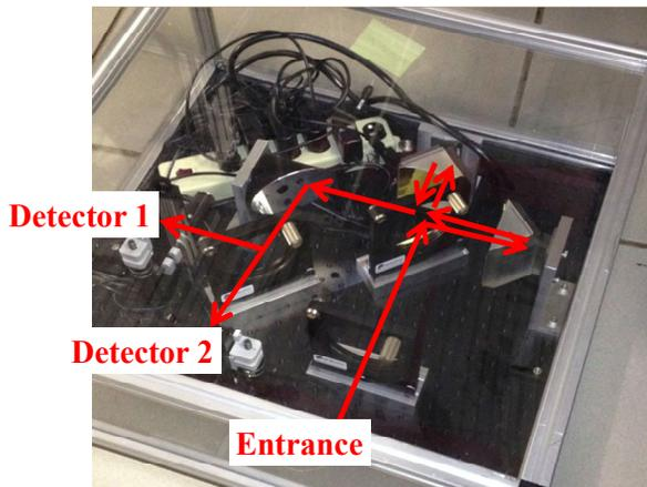
Figure 14: Interferometer light path. The THz is split and recombined from different path lengths. The interference determines the frequency content which in turn determines the bunch length.
