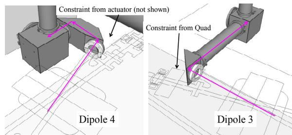
Figure 7: The two compressor source port boxes.
