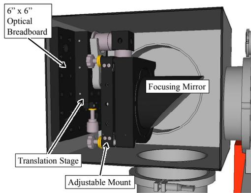
Figure 9: Off-axis parabolic optics in stainless steel box.
