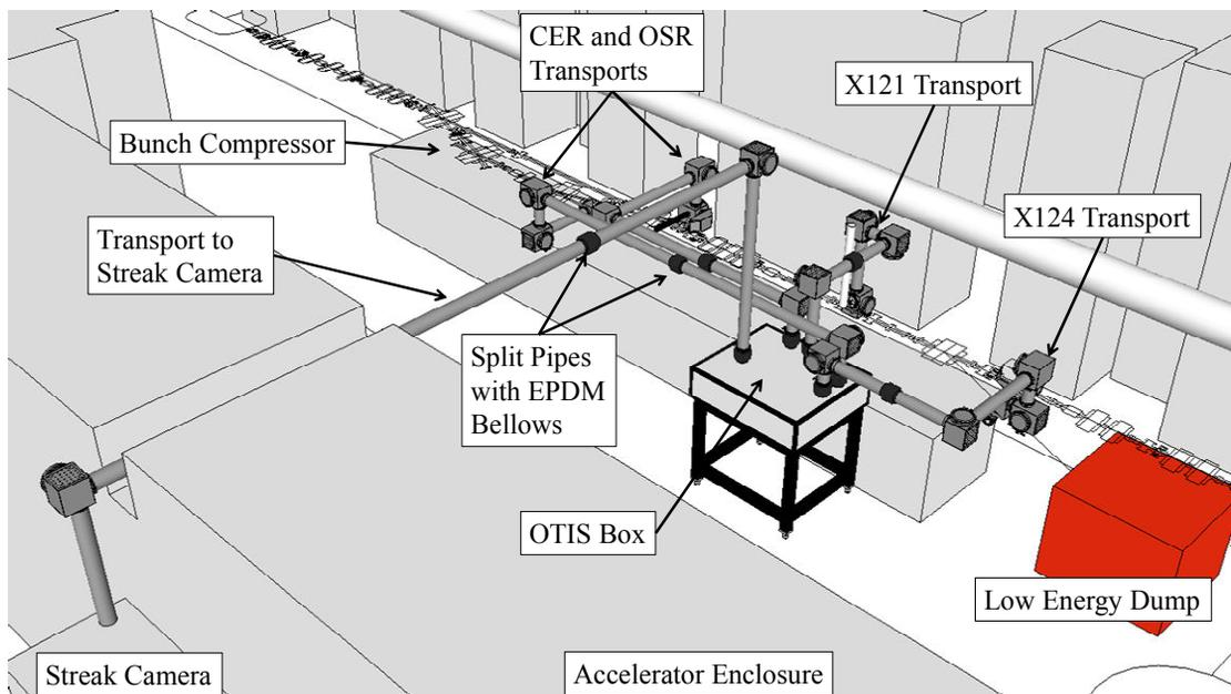
Figure 2: OTIS transport pipes just after the bunch compressor.
