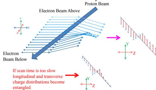
Figure 2: Fast scan of the electron beam through the proton beam. One can see the erf-like deflection from the baseline.
