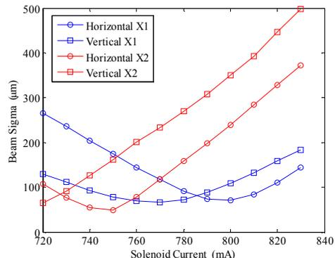
Figure 11: Horizontal and vertical rms beam sizes at the first (blue) and second (red) crosses in the test stand. The electron beam was ~50 keV and 1 μA onto YAG:Ce screens.
