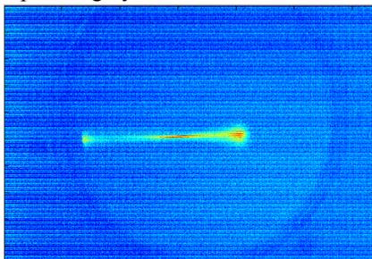
Figure 13: Trace of the electron beam on the phosphor screen for a deflecting voltage of ~150 V. This image was not taken with the design optics. It was taken with just a camera and objective lens. The beam started off the screen on the left side and was then swept to the right.
