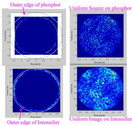
Figure 16: Ray tracing from source (top) to image planes (bottom) to determine aperture (left) and uniformity (right).
