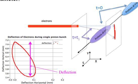
Figure 3: Trajectory followed by a stationary electron beam as the proton bunch passes by. There is some deflection along the proton beam direction due to the magnetic field of the proton beam, but it is much smaller than the deflection transverse to the proton beam.
