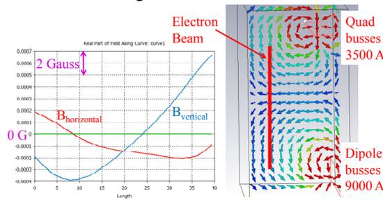
Figure 17: CST simulation of magnetic field from magnet busses along the line of the electron beam. The horizontal component is most important as the electron beam is vertical. The maximum horizontal field is 2 G.
