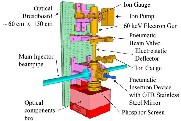
Figure 5: Model of the EBPs showing the main components.
