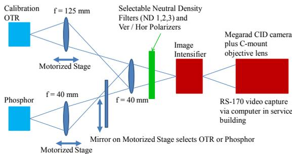
Figure 8: Optical paths followed by the OTR light and the phosphor screen light. Of the two lenses in each path, one is shared.
