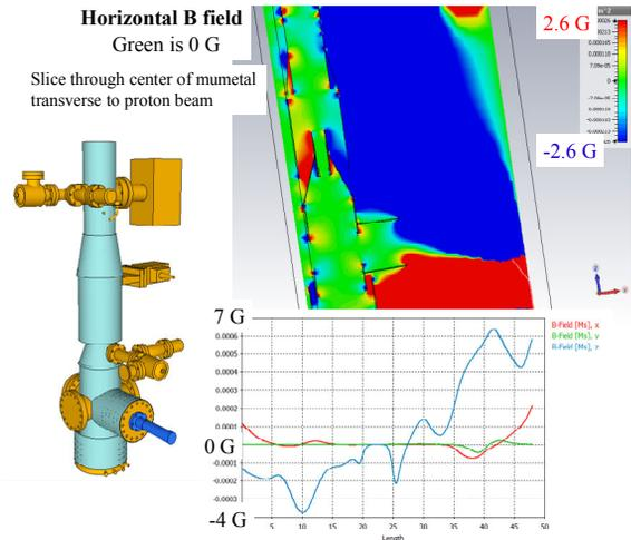
Figure 18: Model of mumetal wrap. The intensity plot is a CST simulation of the magnetic field inside the mumetal shield. The residual horizontal fields (red and green in the lower plot) are significantly less than 1 G with the exception of the ends.
