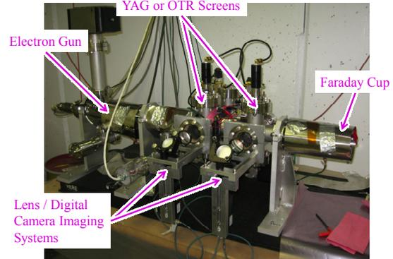
Figure 10: Initial test stand for measuring beam parameters.
