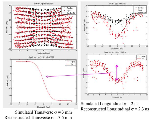
Figure 15: Simulated deflection data for varying impact parameters. The black points are baseline deflections with no beam. They result from the non-uniform deflector field. Each point represents a single electron with the random spread given by the measured emittance.
