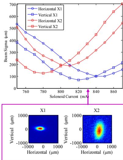
Figure 12: Horizontal and vertical rms beam sizes at the first (blue) and second (red) crosses in the test stand. The measurements are from OTR taken at ~50 keV and 1 mA beam current onto the stainless steel mirrors.
