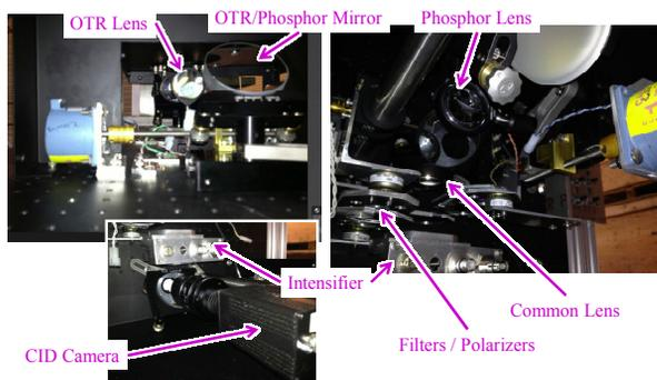
Figure 9: Optical components mounted inside box. The top left picture is looking vertically along the OTR line. The top right picture shows the phosphor path.
