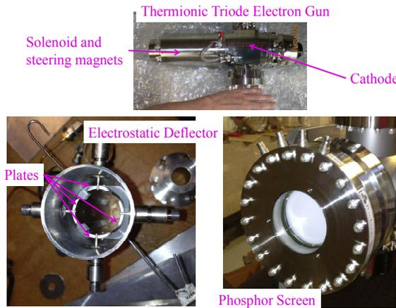
Figure 7: Left) Inside view of the electrostatic deflector showing the cylindrical parallel plates. Right) Phosphor screen mounted in an 8 in Conflat flange. A drain wire is attached between the screen and one of the SHV connectors.
