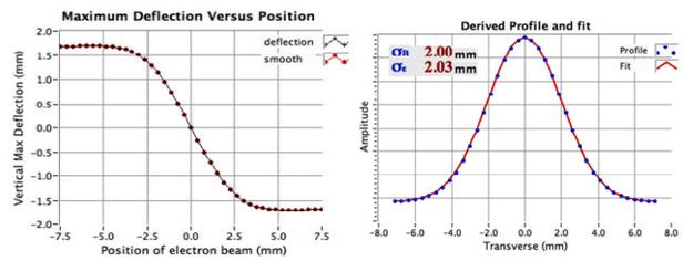
Figure 14: Deflection plot of electron beam, and the derivative of it, showing agreement to better than 2%.
