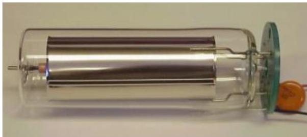
Figure 13: SNS type ionization chamber. [29]
