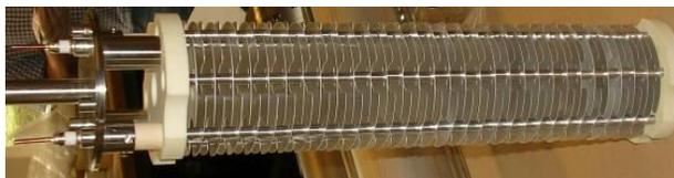
Figure 14: The LHC ionization chamber. [30]
