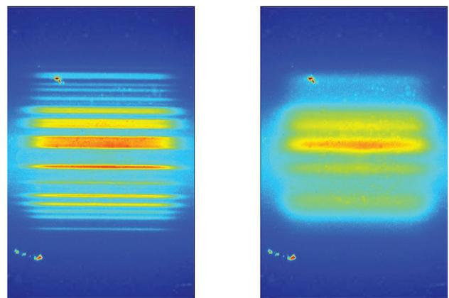
Figure 5: Images of the synchrotron radiation, as viewed through the coded aperture, acquired by the camera. Left: 6.1 μm vertical e<sup>-</sup> beam size,  $\sigma_y$  (0.1 % coupling,  $\kappa$ ). Right: 25.6 μm vertical e<sup>-</sup> beam size,  $\sigma_y$  (1.1 % coupling,  $\kappa$ ).
