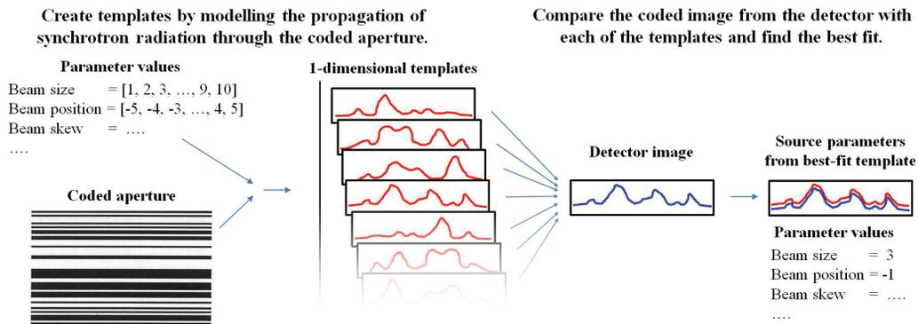
Figure 4: The process used to find the source parameters from the detected image.
