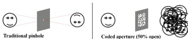
Figure 1: Left: The operation of a traditional pinhole camera. Right: A coded aperture with randomly distributed pinholes, and the resultant overlapping images.
