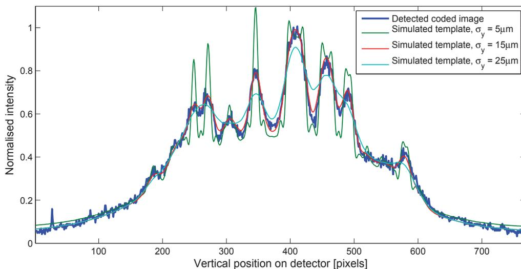
Figure 6: The detected flux for nominal beam conditions ( $\sim 0.3\%$  coupling,  $\kappa$ ) as seen by a single column of pixels from the camera, plotted along with the generated templates for flux seen at each detector pixel for three different vertical source sizes,  $\sigma_y$ .
