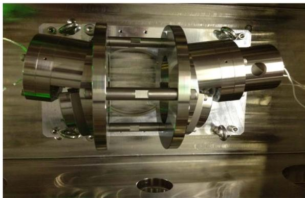
Figure 3: Four mirror cavity.
