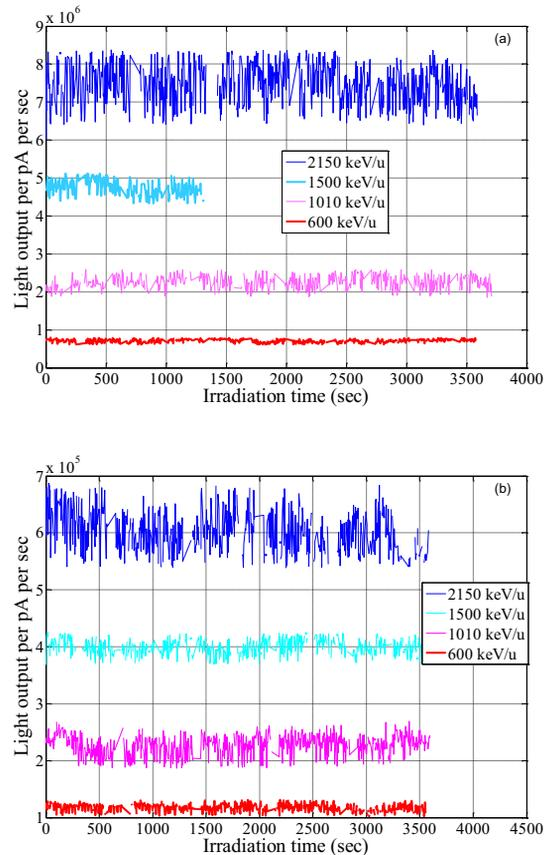
Figure 3: Light yield of (a) CsI:Tl and (b) YAG:Ce as a function of irradiation time at H<sub>2</sub><sup>+</sup> beam energies of 600-2150 keV/u.
