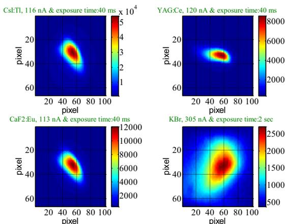
Figure 2: The initial beam spot image on CsI:Tl, CaF<sub>2</sub>:Eu, YAG:Ce and KBr under H<sub>2</sub><sup>+</sup> irradiation at the beam energy of 2150 keV/u.
