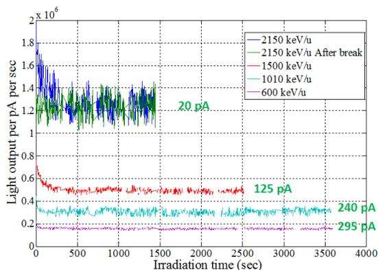
Figure 4: Light yield of  $\text{CaF}_2:\text{Eu}$  as a function of irradiation time at  $\text{H}_2^+$  beam energies of 600-2150 keV/u. For 2150 keV/u, after 24-min irradiation (blue curve), a 10-min break was applied and followed by 24 minutes of the second-time irradiation (green curve).
