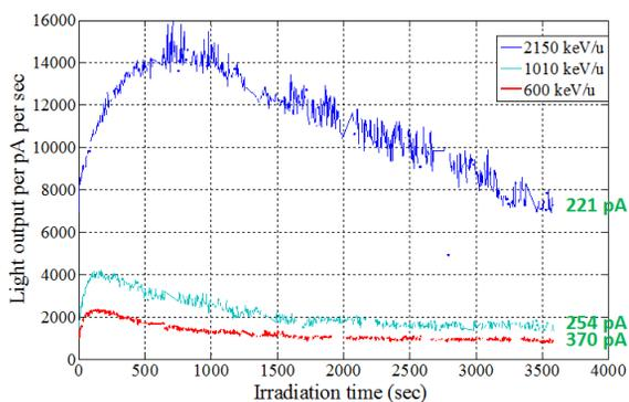
Figure 5: Light yield of KBr as a function of irradiation time at  $\text{H}_2^+$  beam energies of 600-2150 keV/u.
