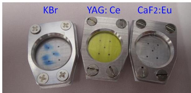
Figure 6: The KBr, YAG:Ce and  $\text{CaF}_2:\text{Eu}$  samples after ion irradiation. The KBr crystal shows damaged spots in blue colour.
