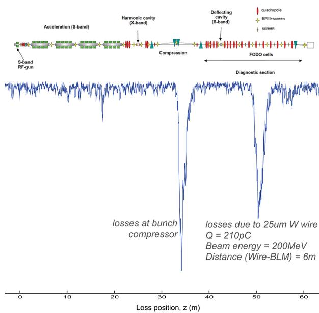
Figure 6: The longitudinal loss monitor uses the arrival time of the Cherenkov photons at the detector to infer the location of the losses.
