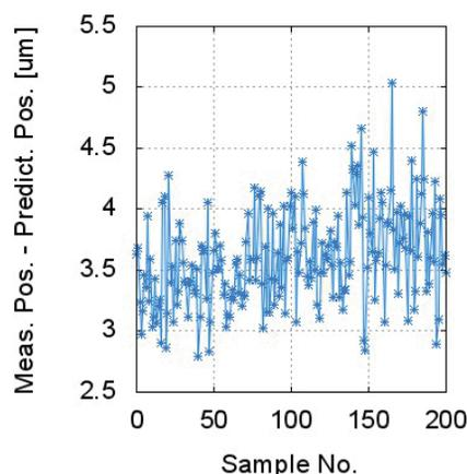
Figure 2: Beam position monitor resolution, measured by comparing several BPMs installed in series.
