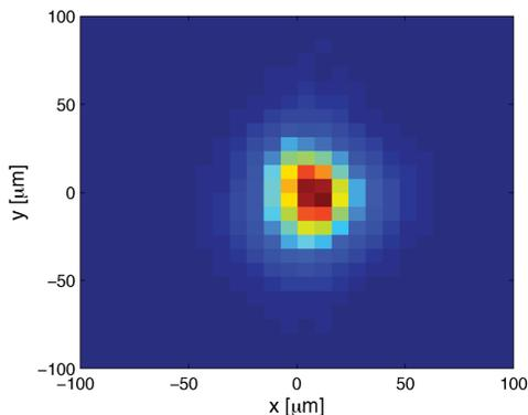
Figure 5: Measurement of a beam with 15 μm rms size.
