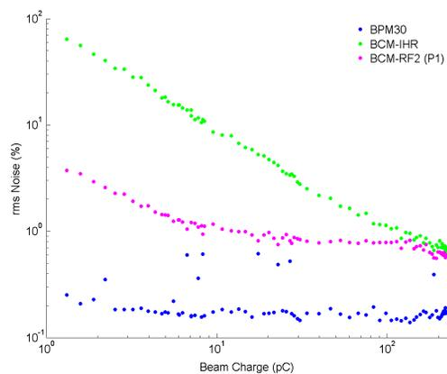
Figure 1: Signal-to-noise ratio measurement as a function of bunch charge, comparing resonant strip line sum signals (BPM30) with charge monitors BCM-IHR and BCM-RF2.
