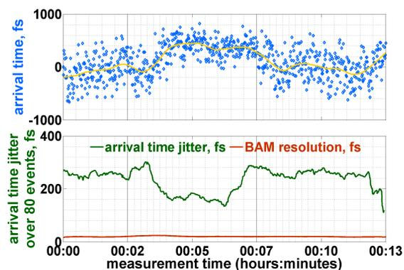
Figure 3: The bunch arrival time monitor has been used to measure arrival time jitter and drift in the SwissFEL Injector Test Facility.
