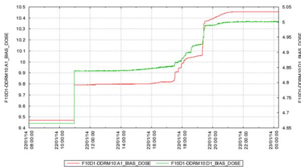
Figure 8: Measurement of dose rate at the undulator installed in Summer 2014. About half of the dose accumulated in this particular day has been deposited during two short time periods, demonstrating the need for a fast interlock system.
