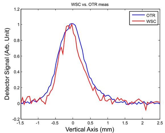
Figure 7: A measurement of beam size with a wire scanner. For comparison, the beam size measured by optical transition radiation is shown.
