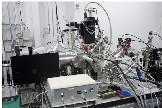
Figure 9: Installation of the terahertz streak camera at SACLA.
