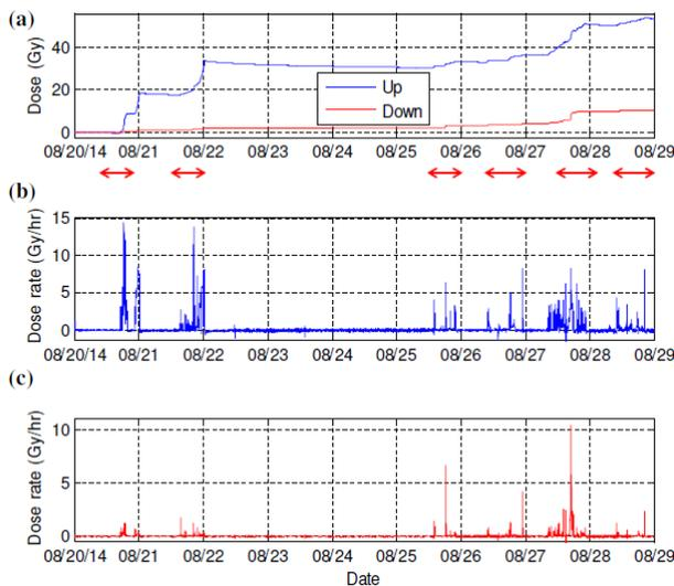
Figure 16: Loss pattern during beam commissioning window from August 20<sup>th</sup> to 28<sup>th</sup>, 2014. The RadFETs are installed at the up side and down side of the vacuum chamber after the injection kicker of the booster synchrotron. The red arrow in (a) is the beam commissioning windows.
