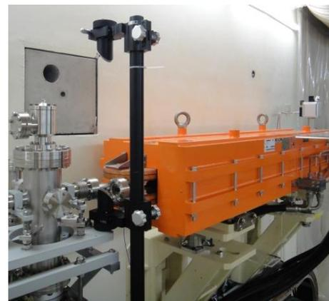
Figure 14: The setup of a synchrotron radiation monitor (SRM) after the 2<sup>nd</sup> BD dipole in the 1<sup>st</sup> cell.
