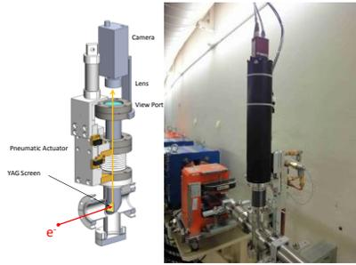
Figure 2: Screen monitor assembly.
