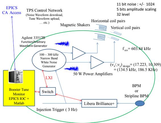
Figure 12: Functional block diagram of the tune monitor.
