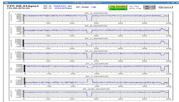
Figure 6: Beam position and intensity trend observed by the 1<sup>st</sup> BPM of the booster synchrotron. The change of the data is caused by the injection condition.
