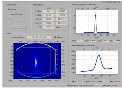
Figure 3: The image profile as the beam passes through the 1<sup>st</sup> screen of the booster ring.
