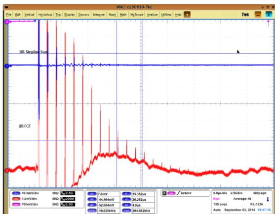
Figure 4: Beam singles observed by a fast current transformer (FCT) and stripline .
