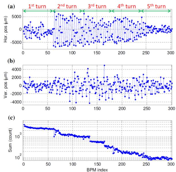
Figure 10: The trajectory in the (a) horizontal plane and (b) vertical plane. (c) Sum signal of the BPMs after aligning the booster chamber and doing the orbit correction.
