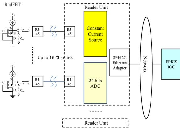
Figure 15: Block diagram of RadFET reader.
