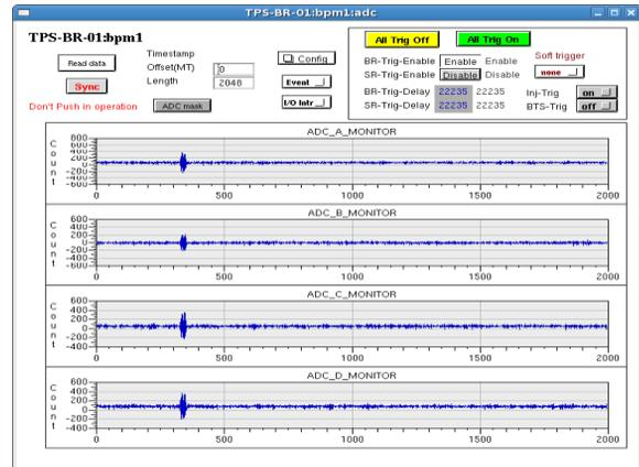
Figure 5: The ADC data when beam passes through the 1<sup>st</sup> BPM of the booster synchrotron.
