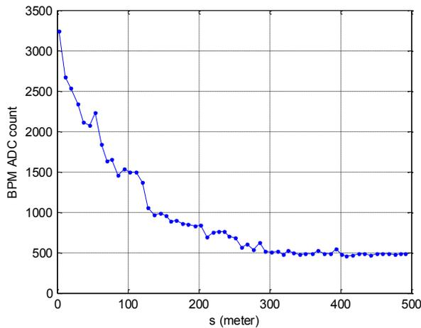
Figure 7: Beam intensity along the booster synchrotron when attempting to circulate the first turn.
