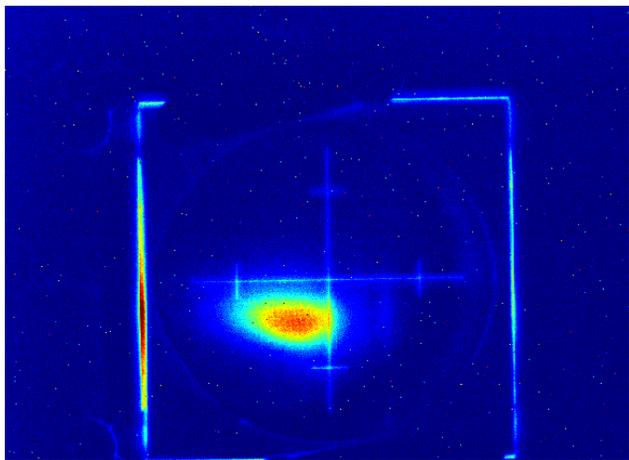
Figure 6: First Lasing at FLASH2. Shown is the spot on the YAG-screen.
