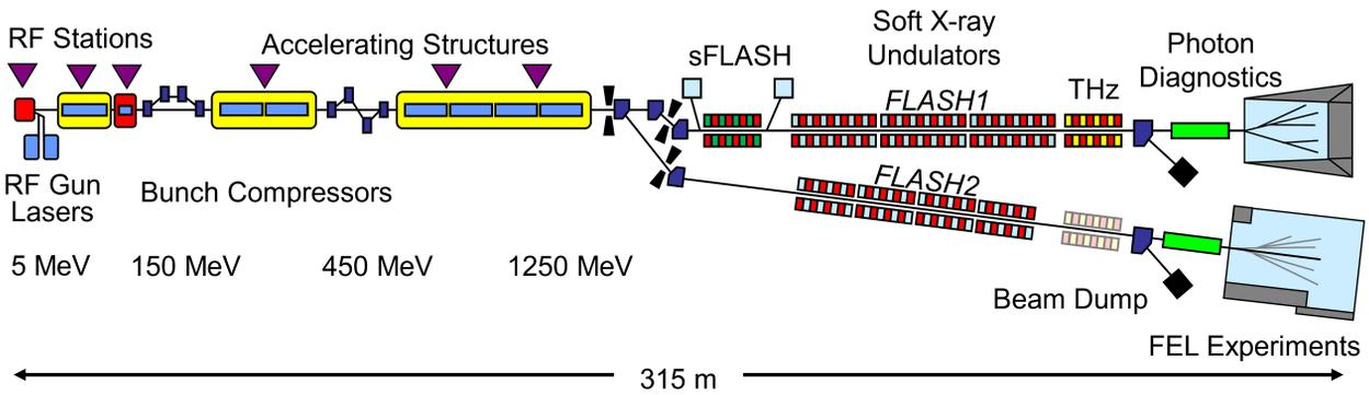
Figure 1: Schematic layout of the FLASH facility. The electron gun is on the left, the experimental hall on the right. Behind the last accelerating module, the beam is switched between FLASH1, which is the present undulator line, and FLASH2, which is the upgrade.
