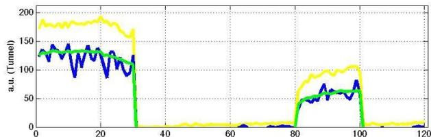
Figure 5: Lasing of two bunch trains with a factor of 2 difference in charge, e.g. of 0.5 nC for the first and 0.25 nC for the second bunch train. The horizontal scale is  $\mu\text{s}$ . The blue line indicates the actual SASE pulse energy produced by each individual electron bunch in the macro pulse. The green line is the time average of this signal. The yellow line indicated the maximum SASE level which occurred since the measurement was started.
