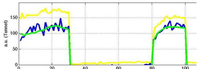
Figure 3: Lasing of two bunch trains with the same charge of about 0.5 nC. The horizontal scale is  $\mu\text{s}$ . The blue line indicates the actual SASE pulse energy produced by each individual electron bunch in the macro pulse. The green line is the time average of this signal. The yellow line indicated the maximum SASE level which occurred since the measurement was started.
