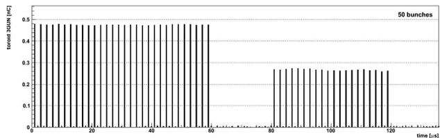
Figure 4: Two trains of bunches, generated by two injector lasers shifted in time.
