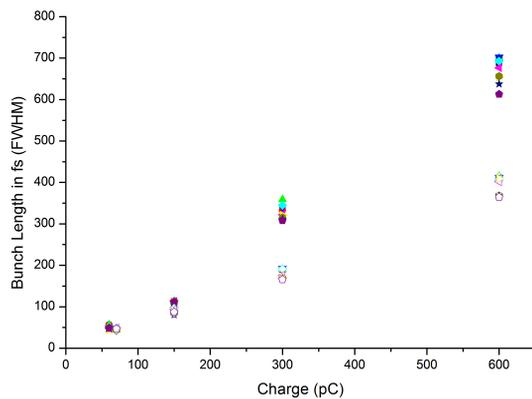
Figure 2: Bunch length for different charges. Measurements have been performed for a beam energy of 0.7 (top) and 1.1 GeV (bottom)
