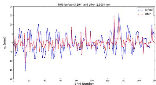
Figure 7: Preliminary test of slow orbit feedback.
