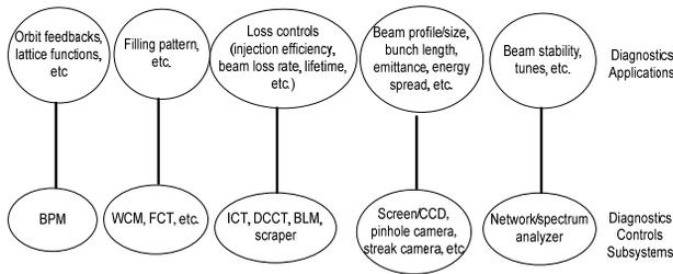
Figure 3: Diagnostics subsystems and applications.
