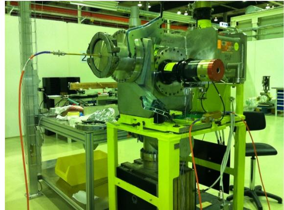
Figure 7: SPS BWS tank with the probe and the hybrid system.
