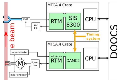
Figure 7: Overview of wire scanner station with corresponding detector readout. Only one motion plane is displayed. The detector can be meters apart from the motion unit.
