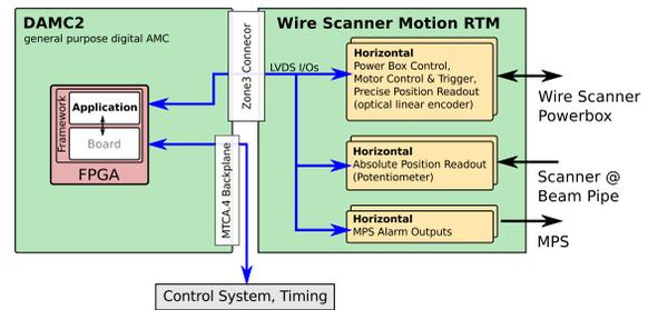
Figure 3: Couple of DAMC2 digital board and wire scanner motion RTM.
