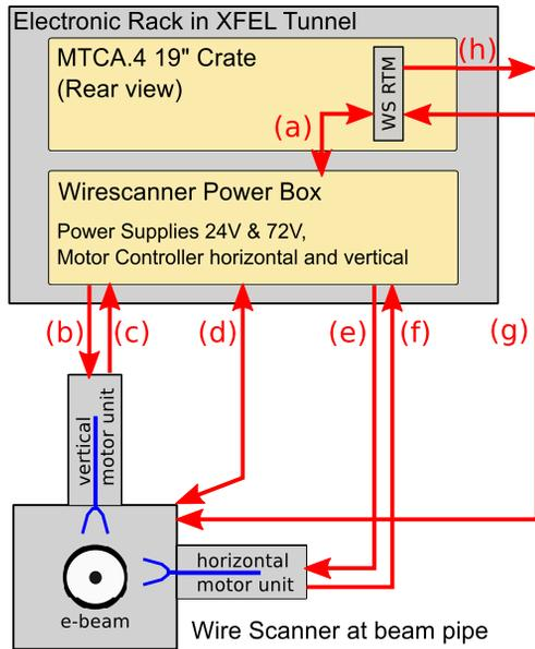
Figure 5: Overview of a complete wire scanner motion unit with RTM to Powerbox cable (a), motor cables (b, e), Heidenhain linear encoder readout cables (c, f), end switches and catch units cable (d), potentiometer readout cable (g) and cable with alarms to MPS (h).
