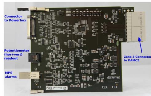
Figure 4: Pre-Series Wire Scanner motion RTM.
