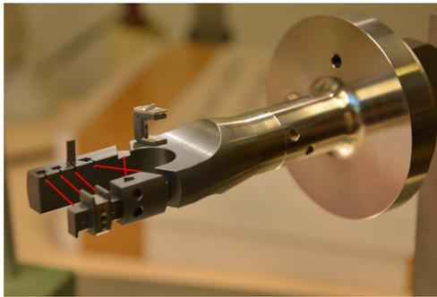
Figure 2: Titanium fork at assembly workstation. Wires are indicated by red lines.
