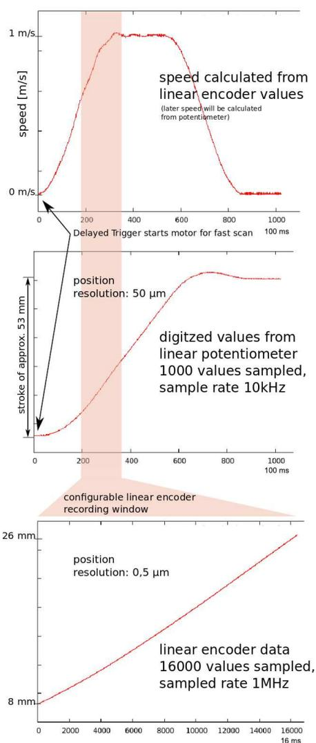
Figure 8: Complete triggered stroke showing speed, linear potentiometer data and high precision linear encoder data.
