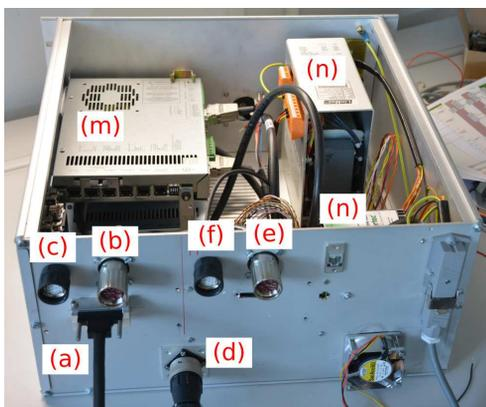
Figure 6: Prototype of Wire Scanner Powerbox (rear view) with LinMot Motor Controllers (m), Power Supplies (n), horizontal and vertical Heidenhain linear encoder readout cables (c, f) and motor cables (b, e), RTM to powerbox cable (a) and cable for end switches and catch units at the scanner (d).
