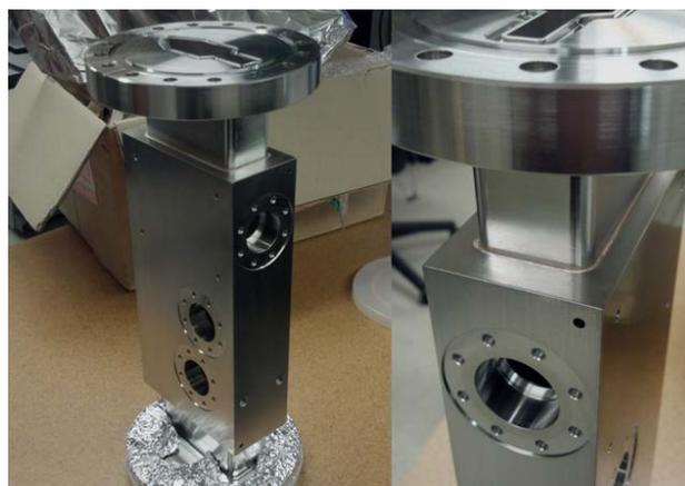
Figure 2: Successfully brazed flag chamber.
