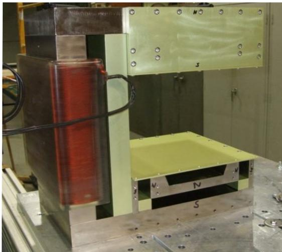
Figure 4: The horizontal detector magnet with the backleg winding.
