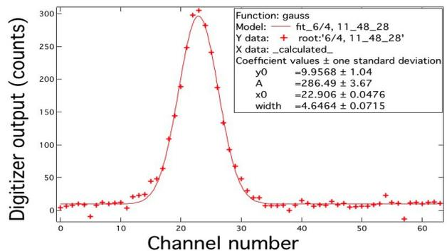
Figure 5: Beam profile during the acceleration ramp.
