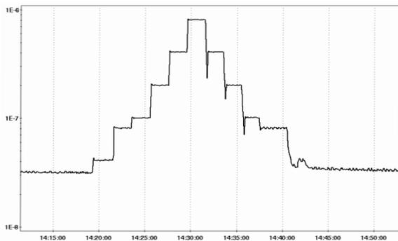
Figure 8: Chamber pressure vs. time for testing of the controlled leak.
