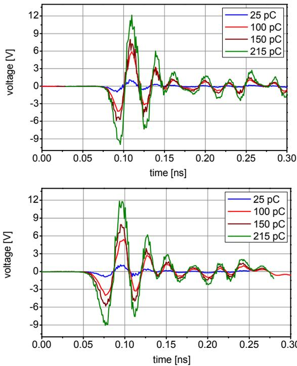
Figure 5: Measured beam pickup signal for bunch charge sweep from 25 pC to 215 pC. Top: Single pickup signal, bottom: combined pickup signal.
