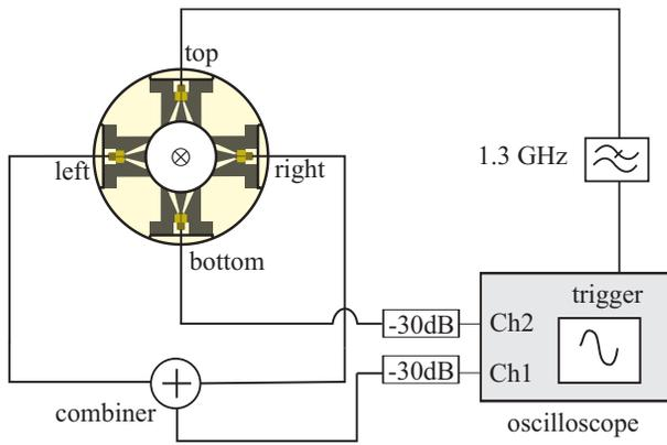
Figure 2: Measurement setup for the time domain measurements of the beam induced pickup signal.
