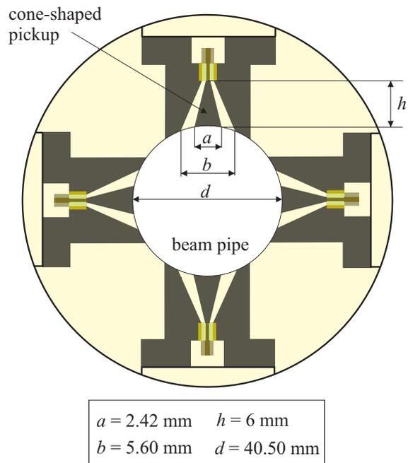
Figure 1: Cross section of the cone-shaped pickup with dimensions [4].
