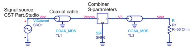
Figure 3: ADS schematics for the RF path simulation. The excitation signal is obtained with a CST PARTICLE STUDIO simulation.
