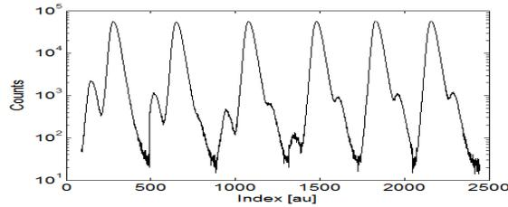
Figure 7: Evolution of double-bucket injection with variable timing between the injector and SPEAR3.
