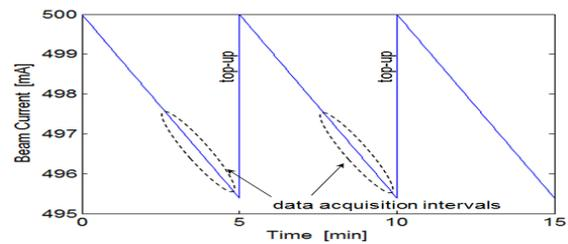
Figure 9: Timing diagram for top-up data acquisition.
