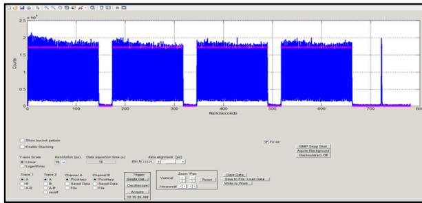
Figure 11: Matlab interface to PicoHarp300 for storage ring bunch pattern analysis.
