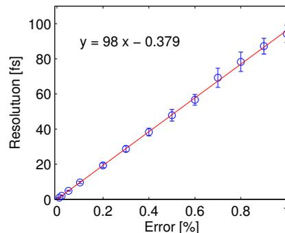
Figure 5: BAM resolution as a function of the signal error. The solid line represents a linear fit.
