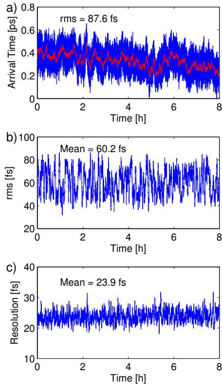
Figure 8: Stability measurement at the bunch charge of 200 pC with optical timing system; a) bunch arrival time, b) bunch arrival time jitter over 100 shots, and c) BAM resolution over 100 shots.
