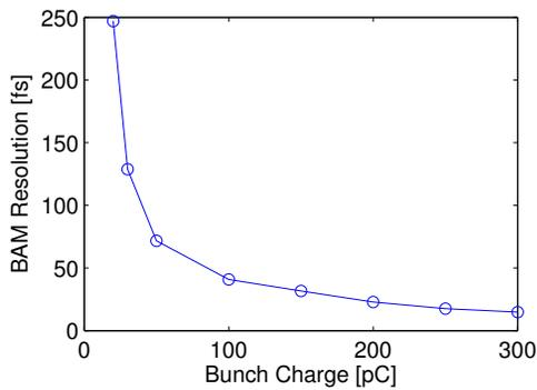
Figure 6: BAM resolution dependence on the charge.
