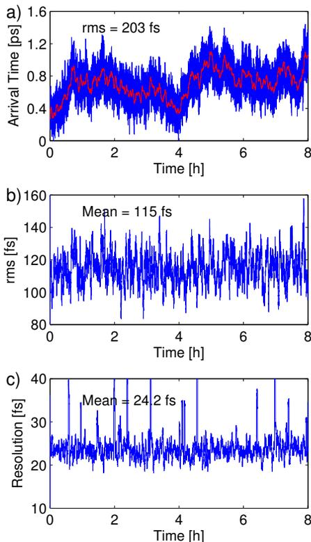
Figure 7: Stability measurement at the bunch charge of 200 pC with RF timing system; a) bunch arrival time, b) bunch arrival time jitter over 100 shots, and c) BAM resolution over 100 shots.
