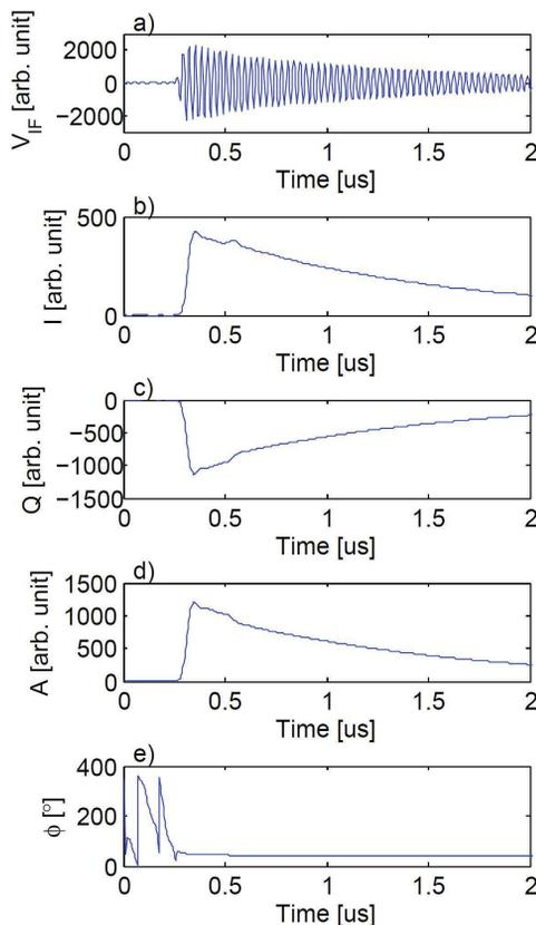
Figure 4: BAM signal processing data for 200 pC bunch charge; a) IF raw data, c) I data, d) Q data, e) amplitude data, and f) phase data.
