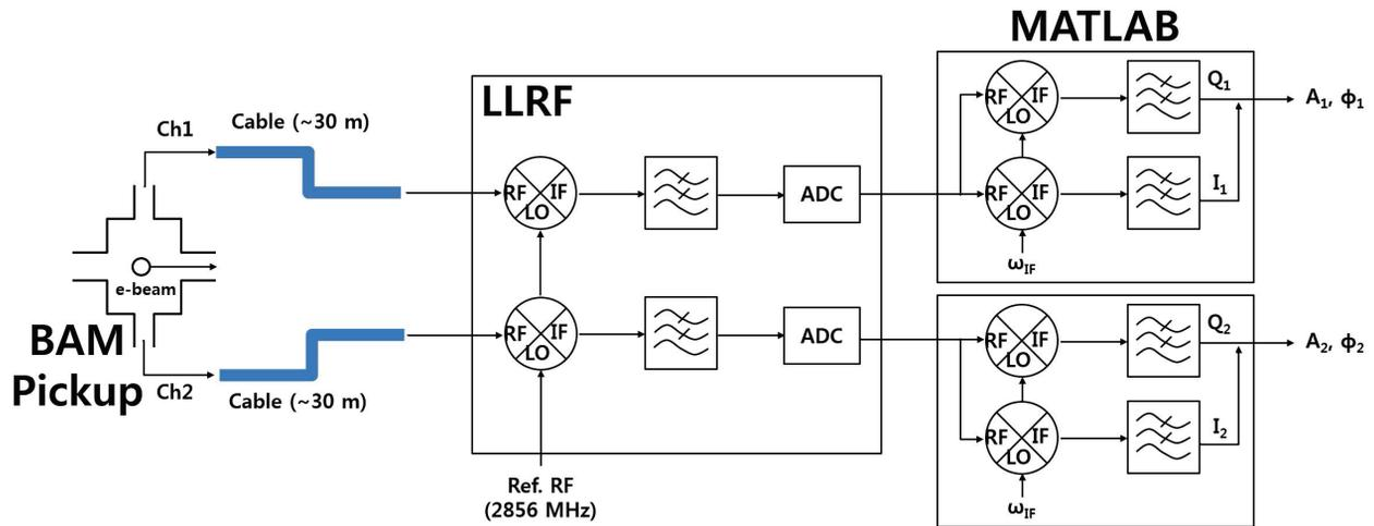
Figure 3: Schematic diagram for signal processing.
