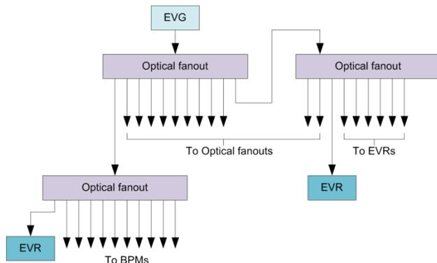
Figure 1: Timing System Event Link Block Diagram.
