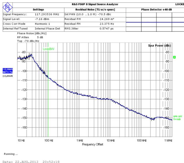
Figure 2: Embedded EVR Phase Noise.
