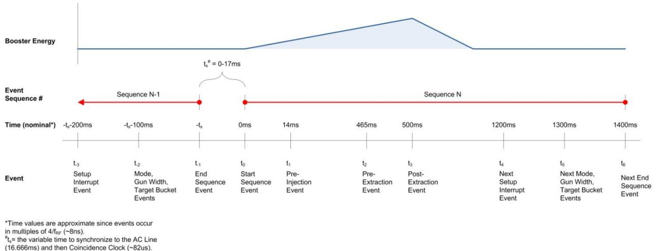
Figure 4: ALS Event Sequence Diagram. The event sequence number and event epochs are shown with respect to relative time and the Booster energy ramp.
