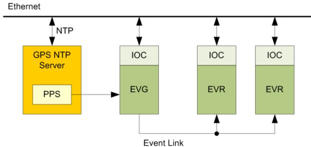
Figure 3: Event System Timestamping Block Diagram.
