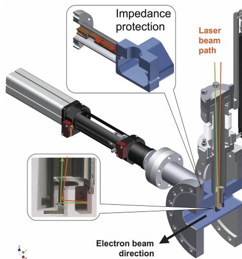
Figure 3: In-vacuum components of the EO-Monitor.
