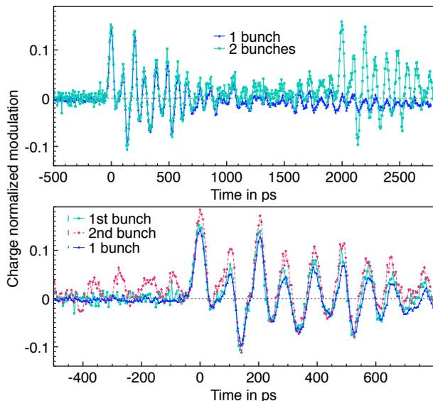
Figure 6: Top: Two EOS scans over a time range of 3 ns. One for a pure single bunch and one for a 2-bunch fill. The EOS-signal is normalized to the charge inside the first bunches. Bottom: Zoom into the region around the first peak for which in addition the signal of the second bunch has been displaced by -2 ns and has been normalized with the charge inside the second bunch.
