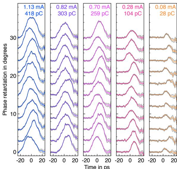
Figure 5: Single-Shot EOSD profiles for different beam currents during one fill ( $V_{rf} = 1.8$  MV,  $f_s = 7.7$  kHz).
