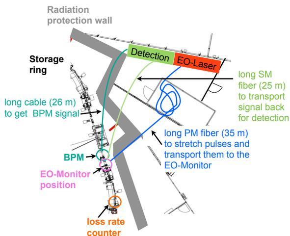
Figure 2: Near-field EOSD setup at ANKA.
