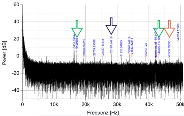
Figure 2: Bunch arrival time readout in frequency domain for a 101 kHz beam at 76 pC.
