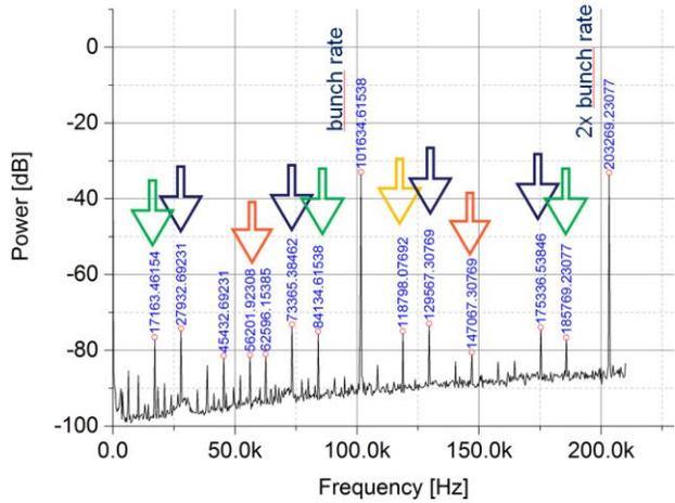
Figure 4: Power spectrum of the broadband THz source.
