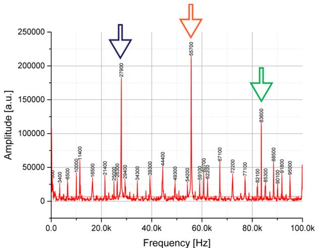
Figure 7: High voltage ripple in frequency domain. The measurement is dominated by 28 kHz and harmonic spurs
