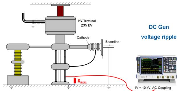
Figure 5: Schematic of the DC gun's high voltage terminal.
