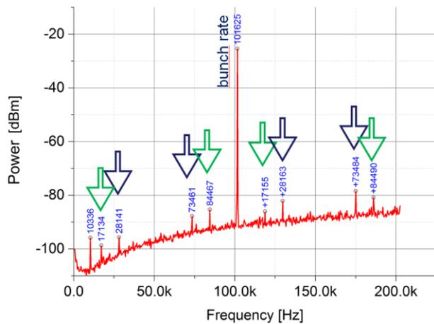
Figure 3: Power spectrum of the BPM readout. The 101 kHz carrier generated by the beam is modulated with repetitive spurs.
