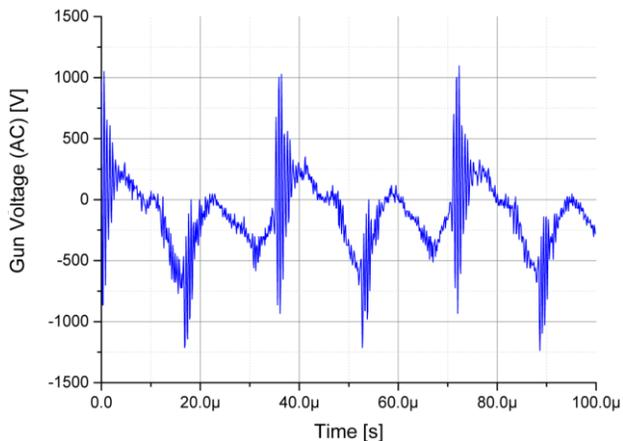
Figure 6: High voltage ripple in time domain with a 56 kHz sine component and bursts at 28 kHz rate.
