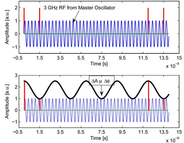
Figure 2: Conceptual representation of the modulated vs. non modulated laser pulses.
