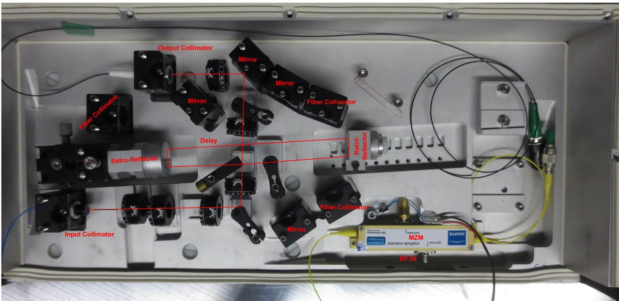
Figure 4: Commission process of the opto-mechanical setup for the novel synchronization system.
