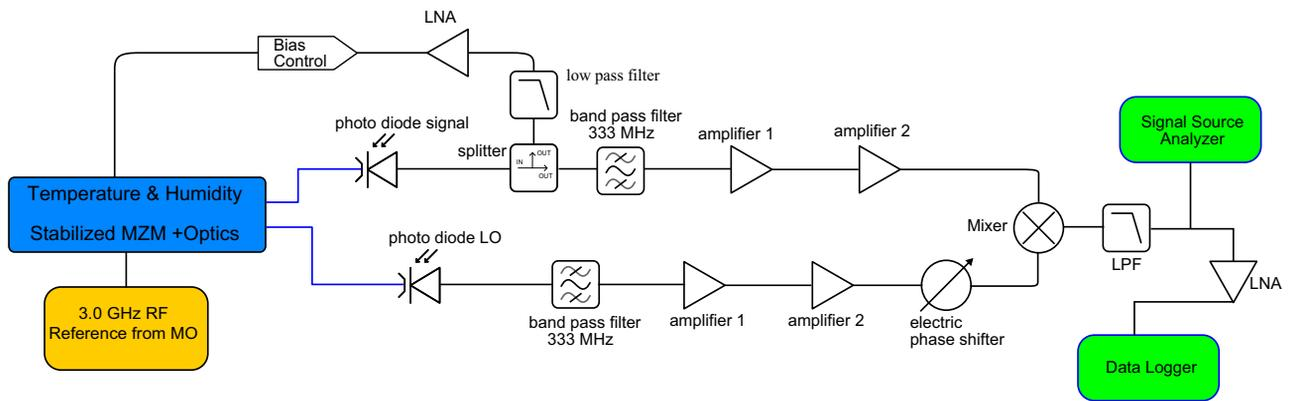
Figure 6: Schematics for amplitude modulation read-out electronics.
