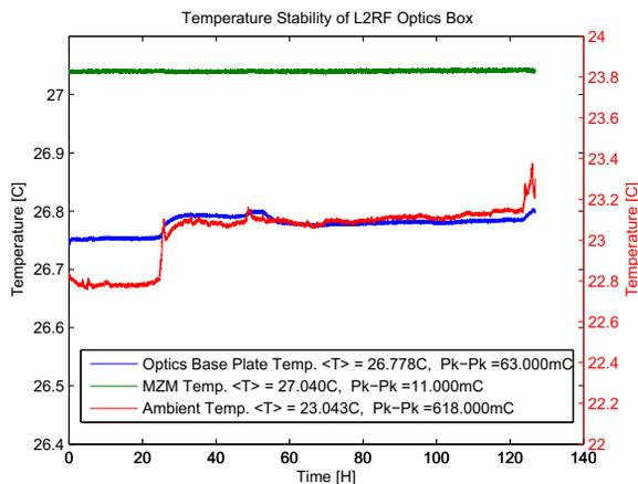
Figure 5: Temperature stability of the engineered baseplate.
