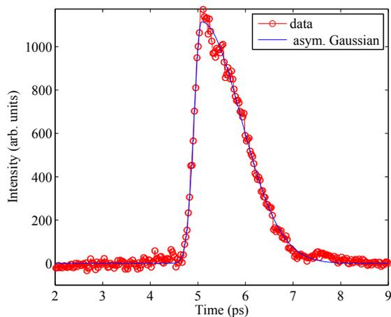
Figure 7: Bunch profile acquired with the GaP 0.1 mm crystal (in red) and asymmetric Gaussian fit (in blue).
