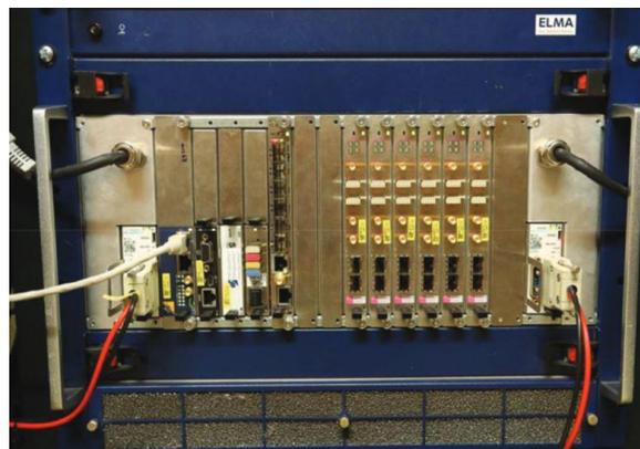
Figure 1: MTCA.4 crate equipped with AMC cards.
