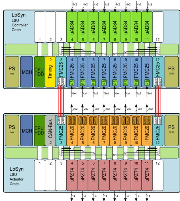
Figure 3: MTCA.4 setup for controlling up to 32 LSUs.
